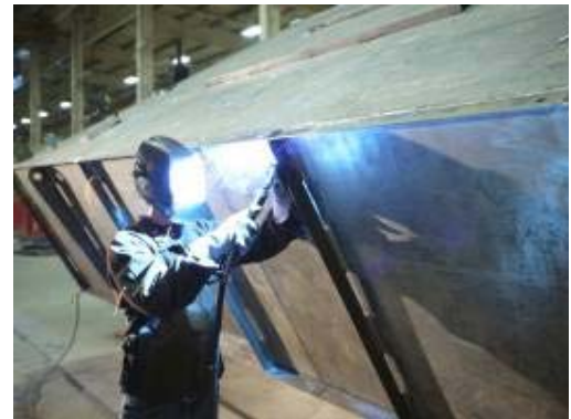
Final welds of a TPS UL Sub Base Fuel Ta
