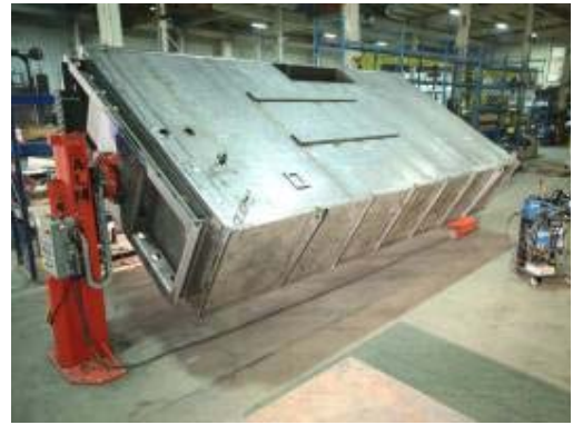
TPS UL Sub Base Fuel Tank getting ready for final welds
