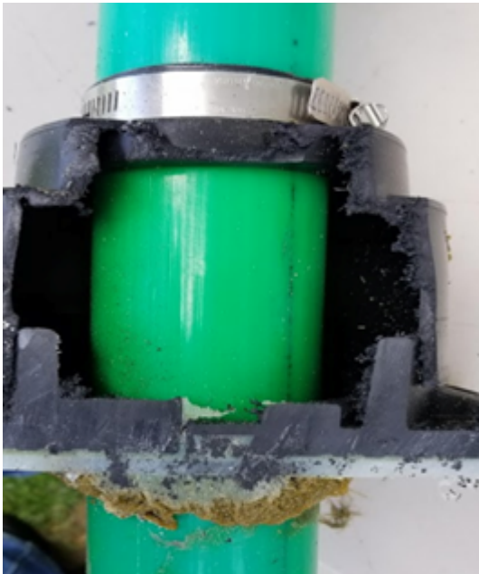
Poly Sump w/Reducer and Test Fittings Photo #18
