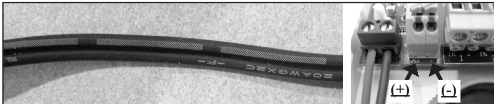
Figure 3—Power Adapter Cable’s White Stripe and the Tank Alarm Console’s Power Connector
