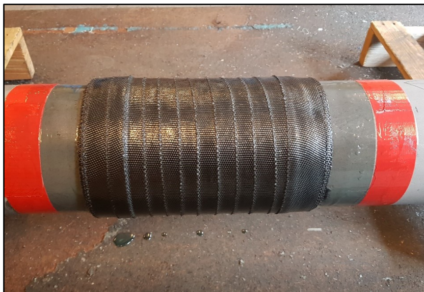
Figure 8: 85% wall loss defect repaired with 10 layers of Revowrap 110 ready for short term survival test
