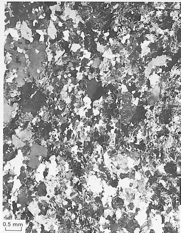
Figures 48a, b. Amerada Petroleum Co., Cowles Magazine No. 2, 12744', St. Lucie Co., Fla. Thin section, ordinary light and crossed nicols, X6.
