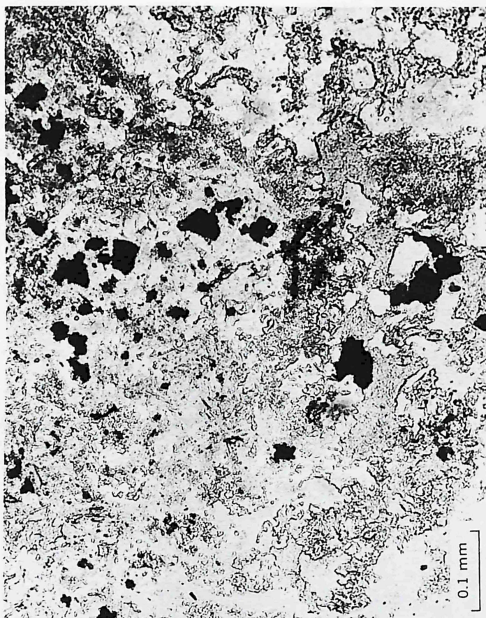
Figure 60. Amerada Swenson No. 1, Okeechobee County, Florida. 10830'-10840' T.D. Hydrothermal quartz (chalcedonic) - chlorite - calcite - ilmenite rock. Ordinary light X150.
