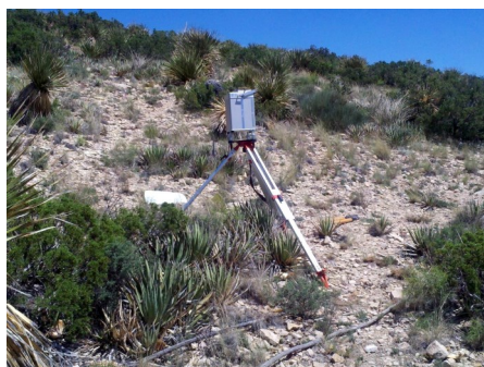
NCKRI photo by Lewis Land CG-5 microgravity meter taking measurements near Manhole Cave.
