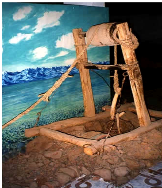
Photograph 1. A windlass is used to bring tunnel spoil to the surface (display at the Qanat Museum in Turpan, China)
