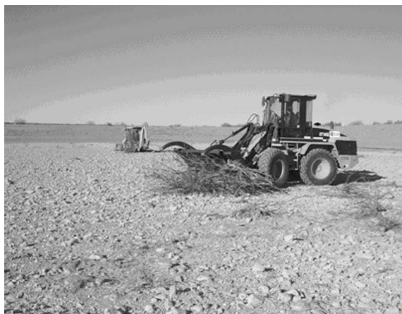
FIGURE 9. IT 14 loader with a brushhog attachment picking up loose tamarisk at LSCR (note the 310 G John Deere backhoe in the background).
