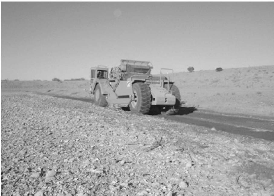
FIGURE 5. 623 CAT elevator (paddle wheel) scraper in Basin 1 at LSCR.
