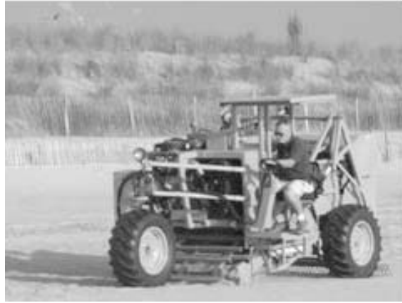
FIGURE 3: Picture of Cherrington Model 5000 Beachcleaner
