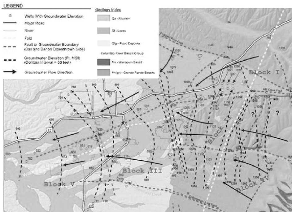
FIGURE 4. Groundwater Flow in Basalt Aquifer System.
