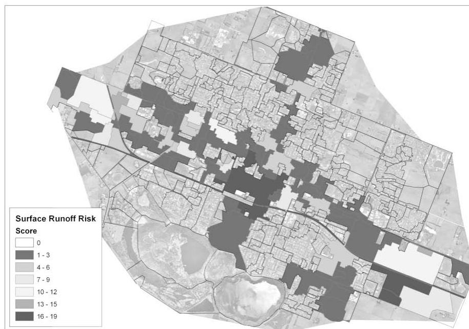
FIGURE 4. Stormwater catchments prioritised by potential contamination from urban land use activities contained in each. Sixteen catchments scored =7 and were at the highest risk of contamination.
