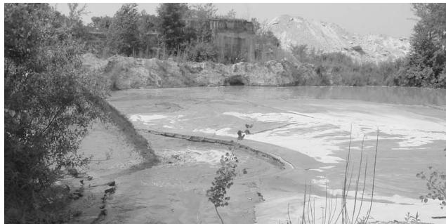
FIGURE 1. Gravel washing in Dover, New Hampshire, for concrete production. Discharge of wash water provides an inadvertent source of artificial recharge to two nearby municipal wells.
