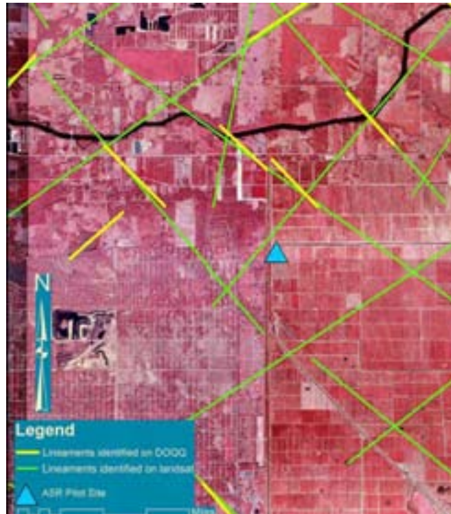
Figure 21. Lineaments identified on DOQQ mosaic in vicinity of Caloosahatchee River ASR pilot site.
