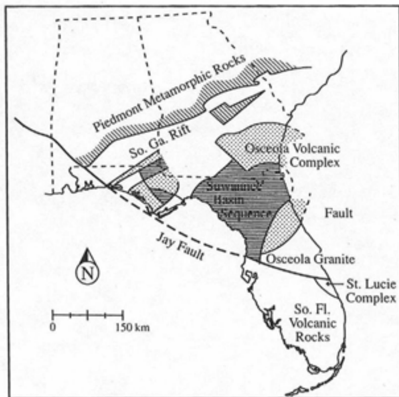
Geologic map of pre-Cretaceous rocks in the basement of Florida and surrounding areas (adapted from Dallmeyer et al. 1987 and Thomas et al. 1989). The Suwannee Basin sequence of undeformed Ordovician to Devonian sedimentary rocks is shown by horizontal lines. The Osceola complex includes the Osceola Granite, the St. Lucie metamorphic rock sequence, and the Osceola volcanic complex (stippled). Where present in the panhandle, the Osceola volcanic complex includes undelineated granitic subcrops. The South Florida volcanic rocks are Mesozoic. The South Georgia Rift area is occupied by Mesozoic sedimentary rocks. The boundary of Piedmont metamorphic rocks is indicated by diagonal lines.
