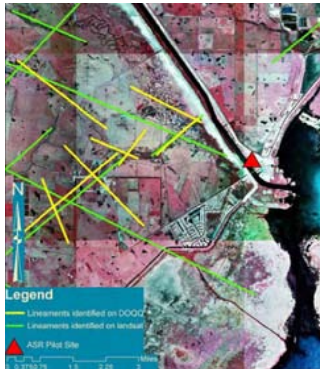
Figure 19. Lineaments identified on DOQQ mosaic in vicinity of Kissimmee River ASR pilot site.
