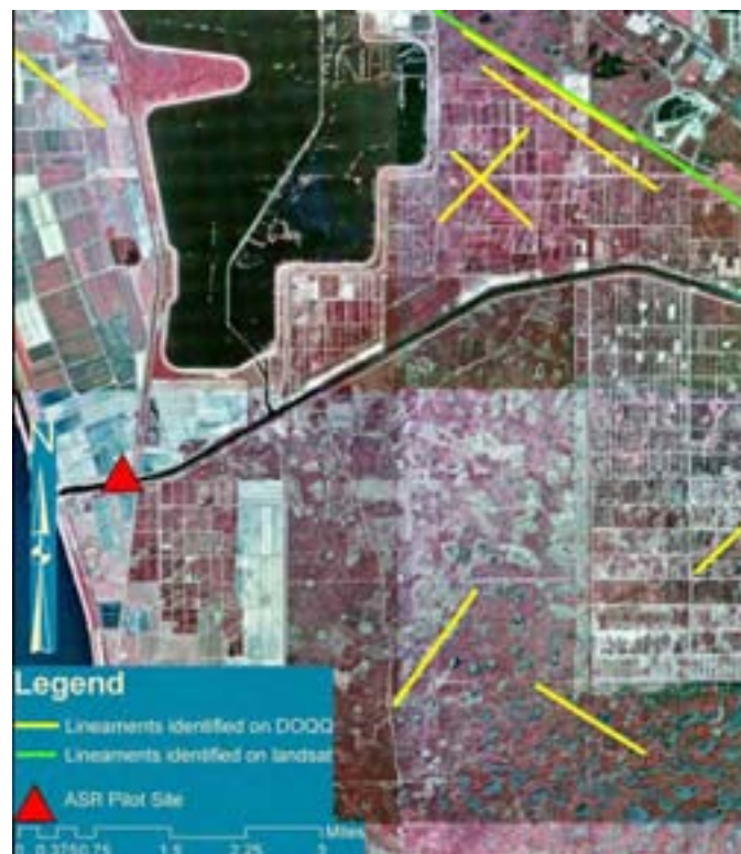
Figure 20. Lineaments identified on DOQQ mosaic in vicinity of Port Mayaca ASR pilot site.
