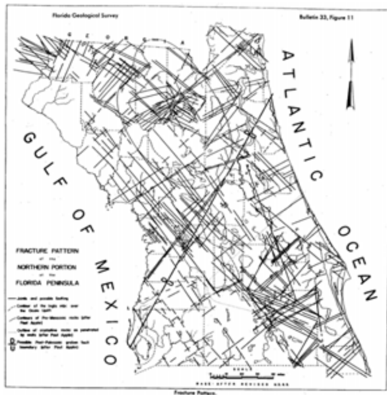
Figure 2. Fracture pattern of the northern portion of the Floridan Peninsula (from Vernon, 1951).
