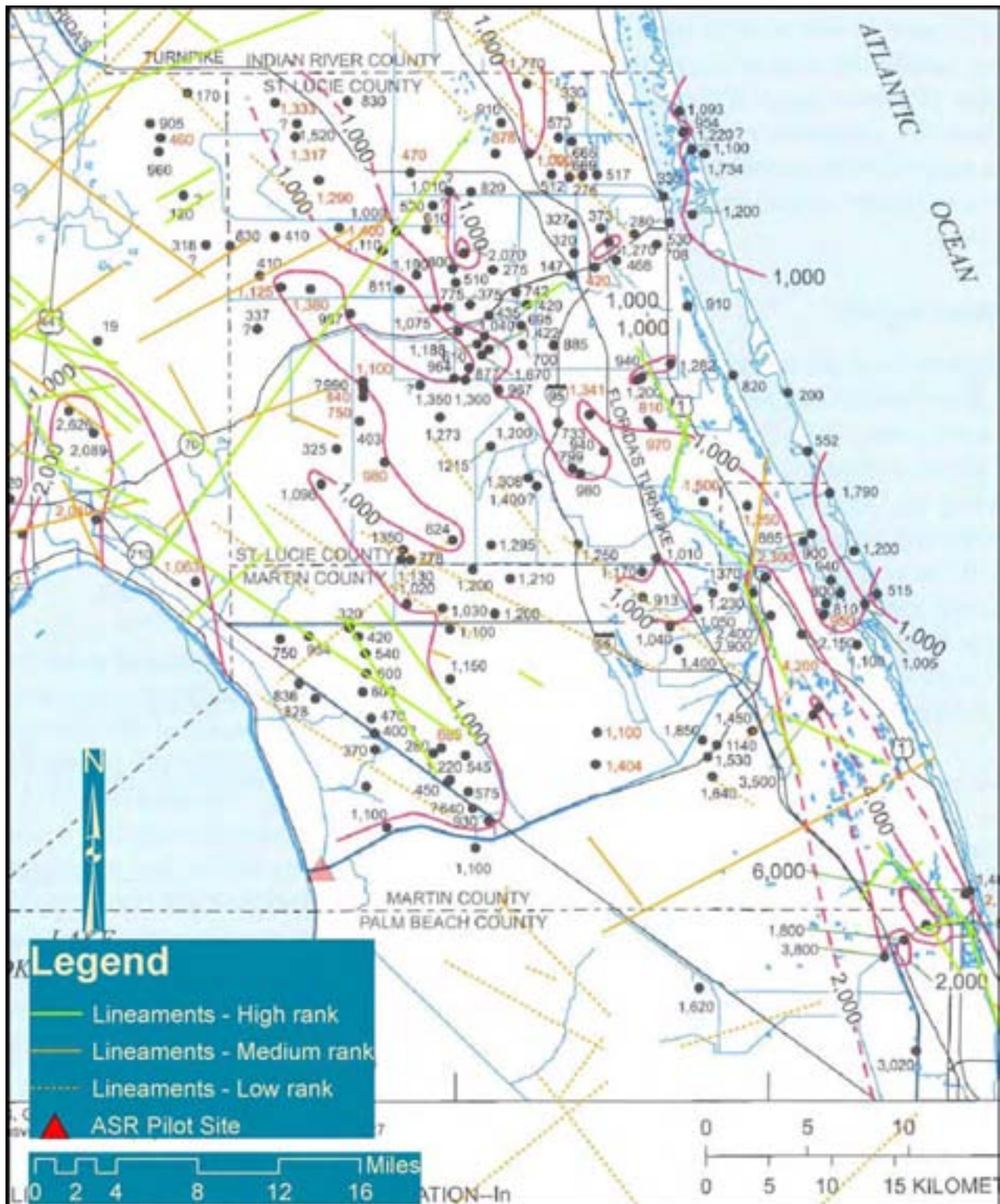
Figure 28. Surface lineaments superimposed on a map showing the distribution of chloride concentration in the Upper Floridan aquifer (modified from Reese, 2004). Contours are lines of equal concentration in milligrams per liter.
