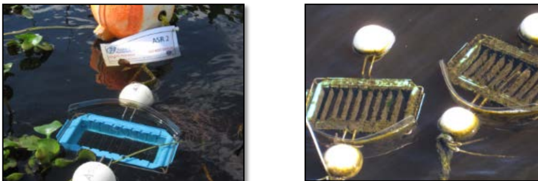
Figure 10-5 – Examples of periphytometers during initial deployment (left), and after a 28-day deployment (right).
