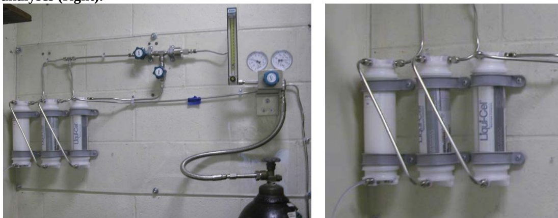
Figure 5. Liqui-Cel TM membrane contactors lab set-up (left) close up of contactors (right).
