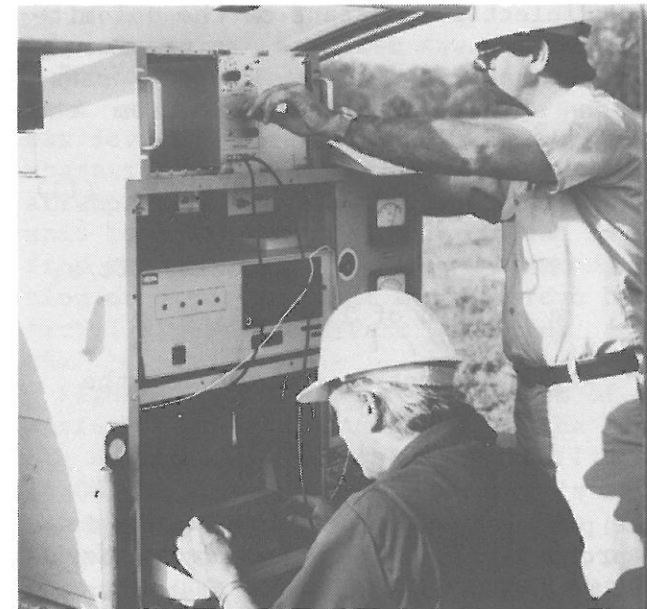
FIGURE 10. - Surface control unit and computer console taking data during scan.
