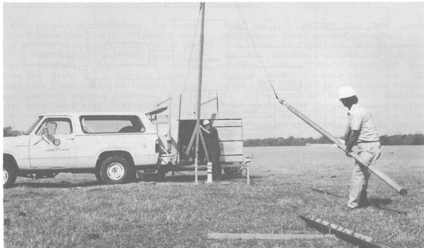
FIGURE 8. - GPR subsurface probe assembly being set up over hole G.
