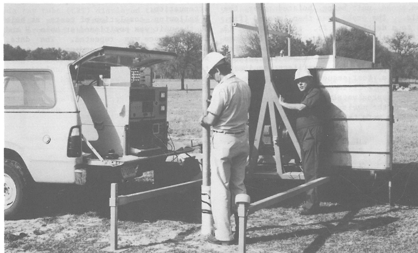
FIGURE 9. - GPR subsurface probe being lowered to a depth of 45 ft.
