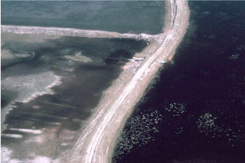
Figure 3. Earthen berms and culvert in the berm that separates the northern and southern sub-basins of Crews Lake in 1971 (upper panel) and 1982 (lower panel) (SWFWMD files). The 1971 photograph also shows a portion of a second berm in the north basin that partitions a portion of the northern sub-basin from the rest of the sub-basin.
