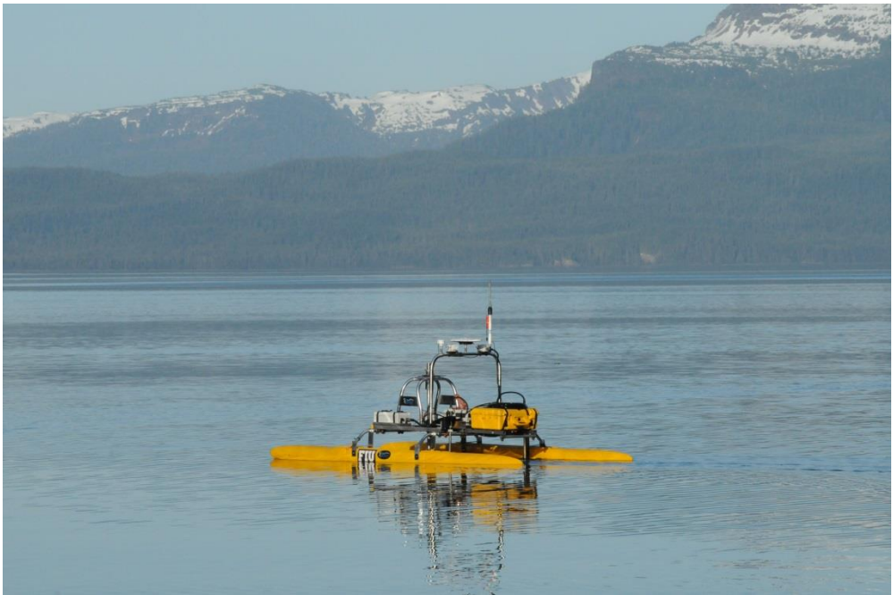
Figure 7: Unmanned surface vessel (USV) in Alaska. It will transit Cudjoe Key lakes and ponds deploying a submersible fluorometer to simultaneously measure dye concentration, and a multi-sensor, water quality monitoring instrument (YSI sonde) to measure physiochemical parameters of water quality.
