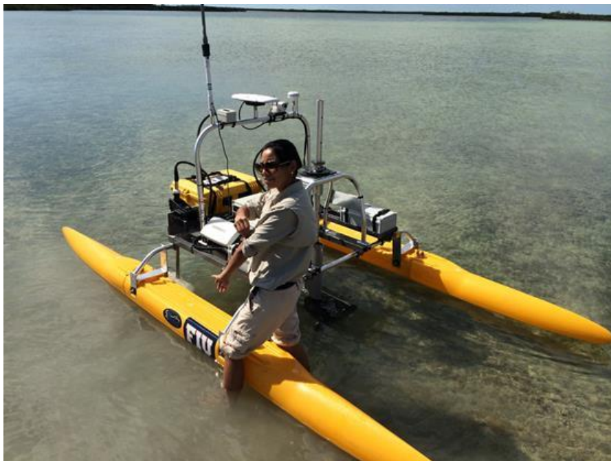
Figure 13: Unmanned surface vessel (USV) in Cudjoe Key deploying a submersible fluorometer to measure dye concentration, and a multi-sensor, water quality monitoring instrument (YSI sonde) to simultaneously measure physiochemical parameters of water quality.
