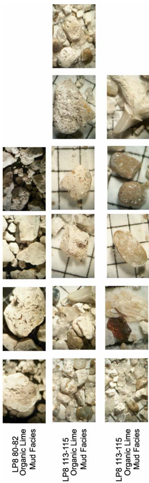
Collage of microscope photographs of grains >1000 microns from the organic lime mud facies in Levys Prairie cores. The core name, sub-sample interval, and respective facies association is on the left and the respective line-up of photos on the right. Backdrop photograph scale is 2mm.
