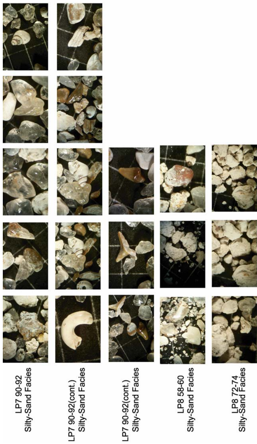
Collage of microscope photographs of grains >1000 microns from silty-sand facies in Levys Prairie cores. The core name, sub-sample interval, and respective facies association is on the left and the respective line-up of photos on the right. Backdrop photograph scale is 2mm.
