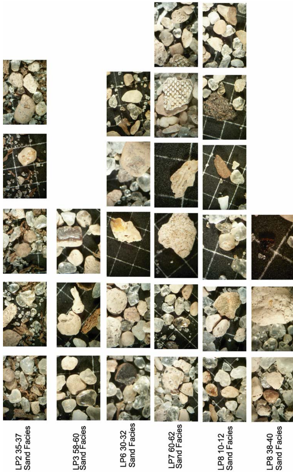
Collage of microscope photographs grains >1000 microns from the sand facies in Levys Prairie cores. The core name, sub-sample interval, and respective facies association is on the left and the respective line-up of photos on the right. Backdrop photograph scale is 2mm.
