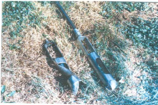
Figure 2. Close-up of stainless steel mud-auger buckets. The right one is undeformed. The left one has been damaged by an attempt to penetrate a zone of refusal.
