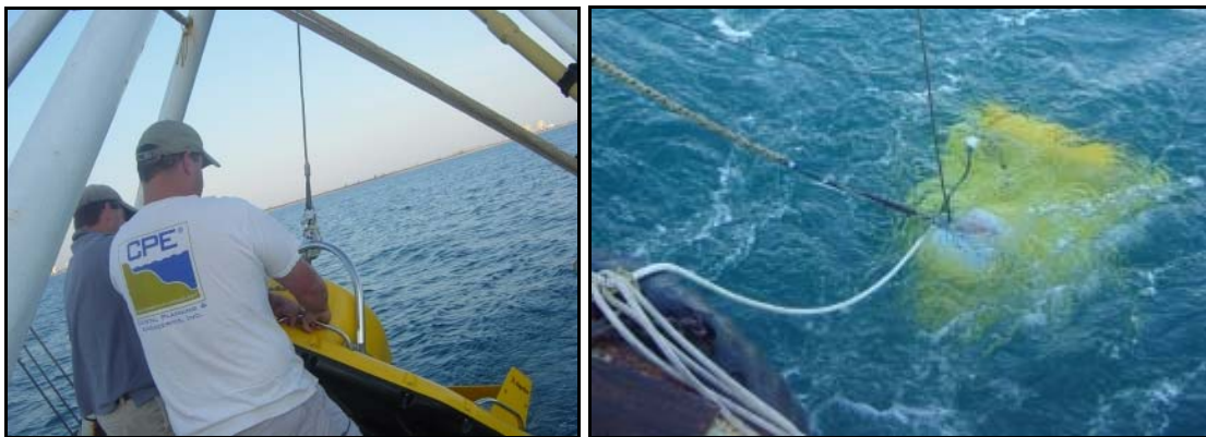
Figure 4. Deployment of the EdgeTech SB-512i sub-bottom profiling system.
