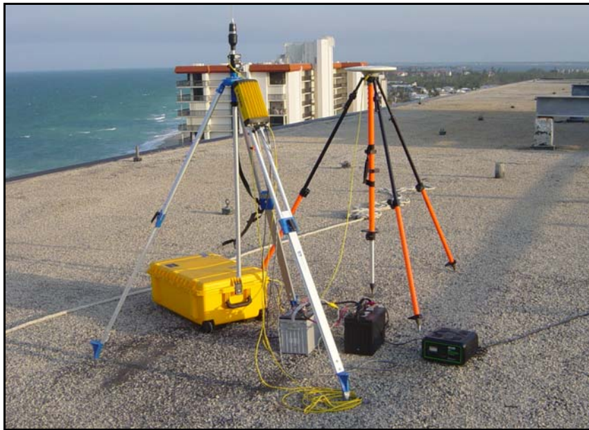
Figure 2. RTK GPS base station “Island Club Base” on the roof of the Island Club Condominiums.
