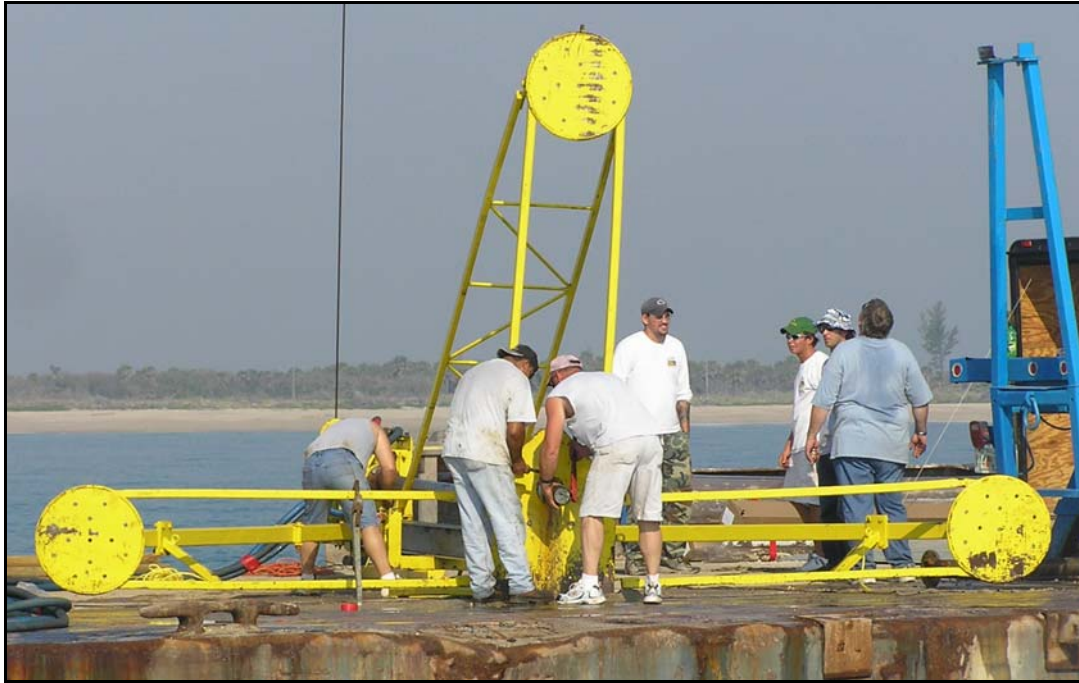
Figure 6. The 271B Alpine Pneumatic Vibracore unit.
