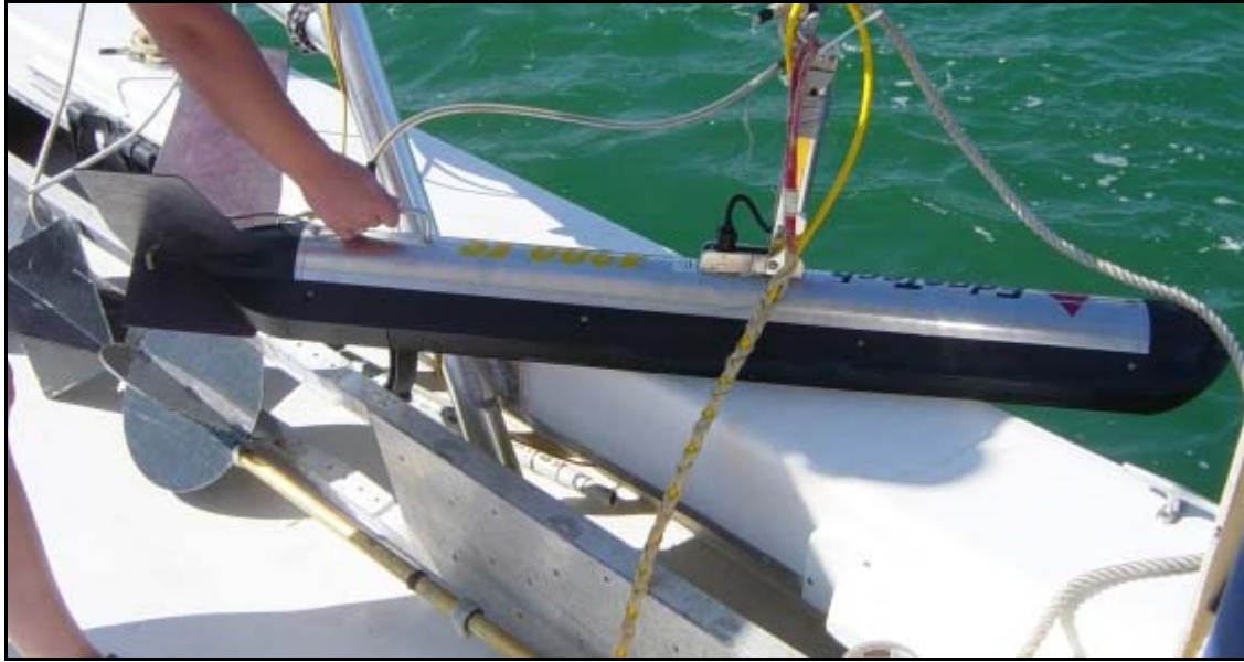
Figure 3. Deployment of the EdgeTech 4200-FS sidescan sonar system.
