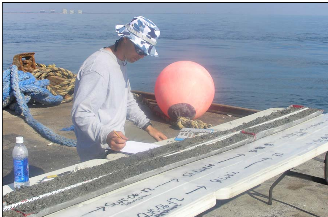
Figure 8. Vibracore splitting, description, sampling, and wrapping being conducted aboard the work barge during the vibracore operations.
