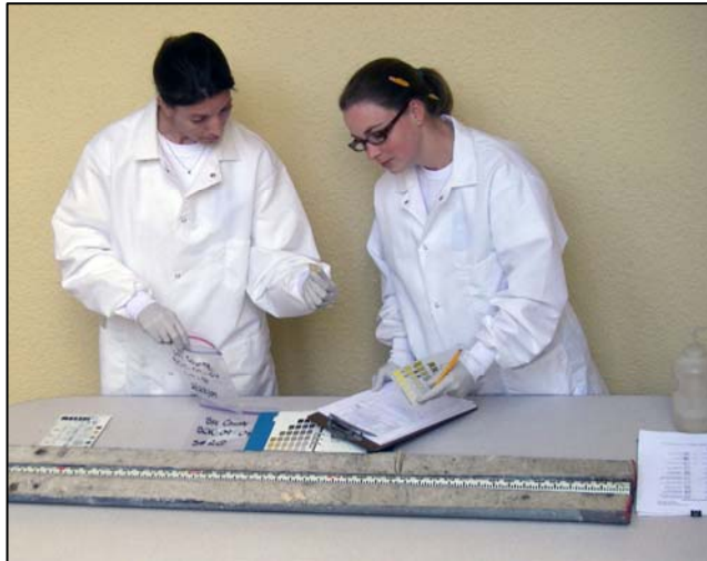
Figure 12. Vibracore logging, sub-sample collection and Munsell color determination being conducted at CPE's office in Boca Raton, Florida.
