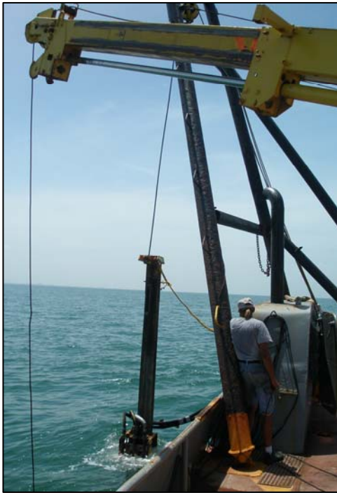
Figure 11. a) Deployment of the 271B Alpine Pneumatic vibracore off the RV Atlantic Twin during the 2008 geotechnical investigation. b) The BH-4 vibracore apparatus being deployed during the 2009 geotechnical investigation.
