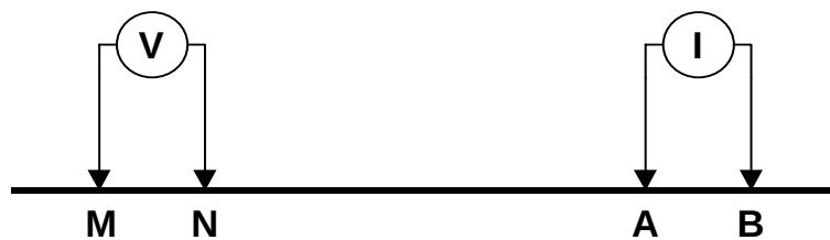
Figure C-2. Standard resistivity electrode geometries.
