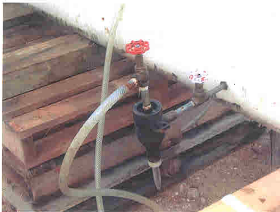
Photograph D-16 - Pumping test Rossum sand sampler
