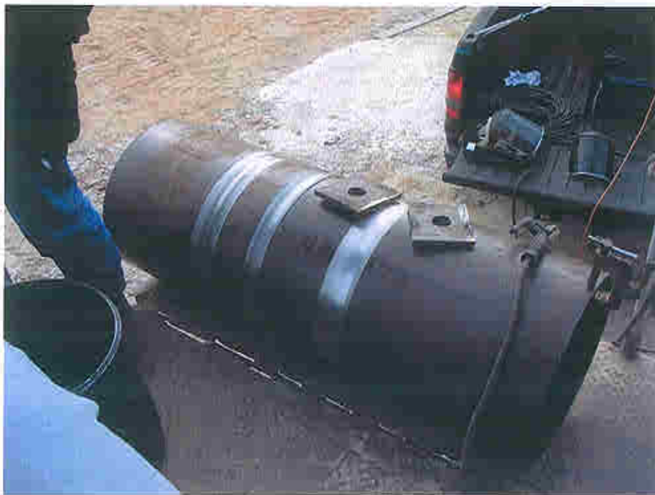
Photograph D-12 - Left-hand back-off casing tool
