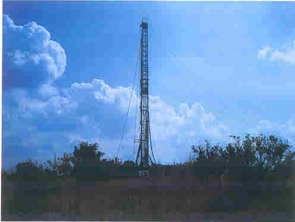
Photograph D-1- Gardner-Denver 3000 trailer mounted drill onsite at Holly Hill LFA Exploratory Well Drill Site.
