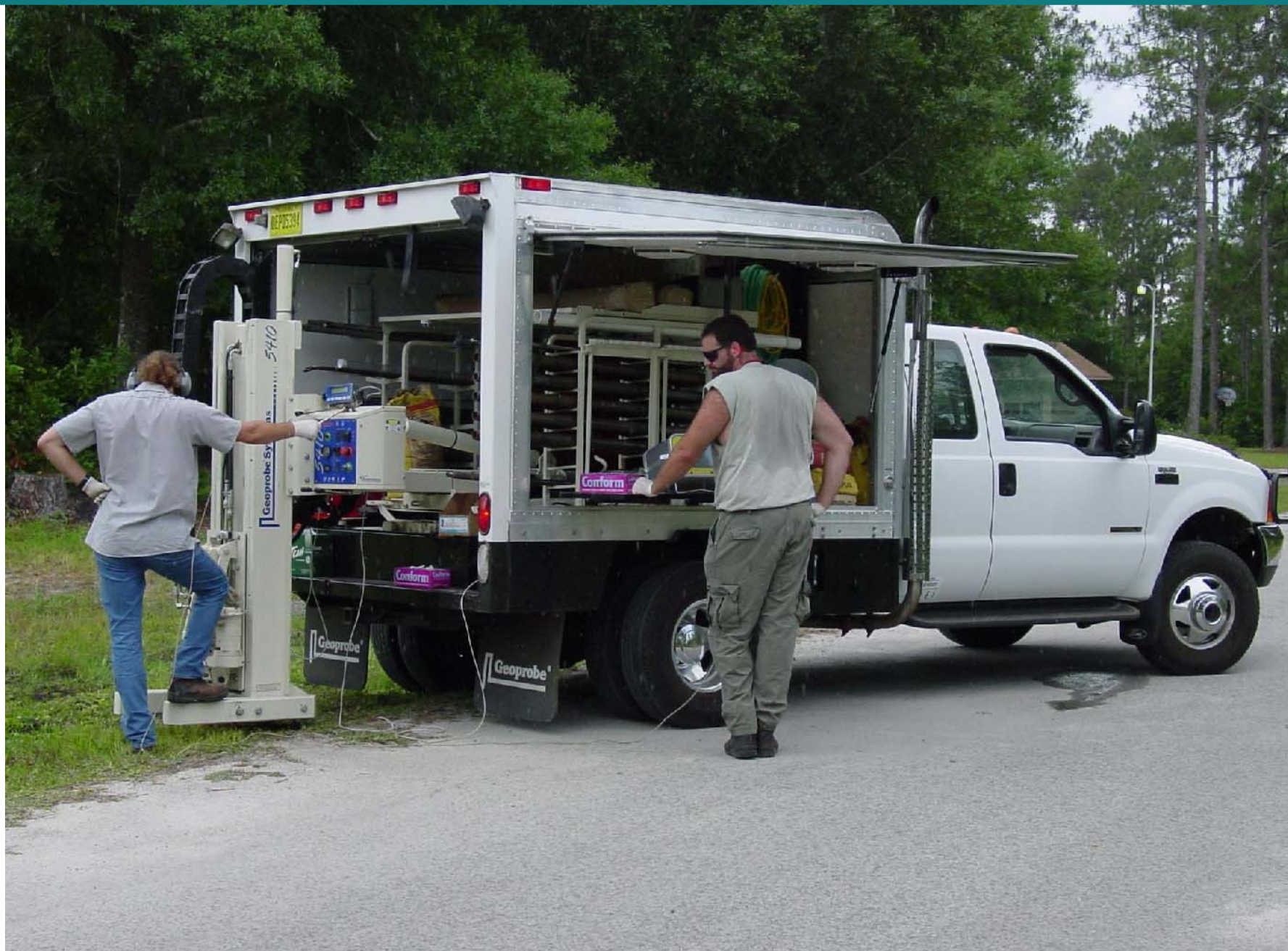
Photograph 4 SIS Direct Push Rig Merritts Mill Pond Arsenic Study Marianna, Jackson County, Florida
