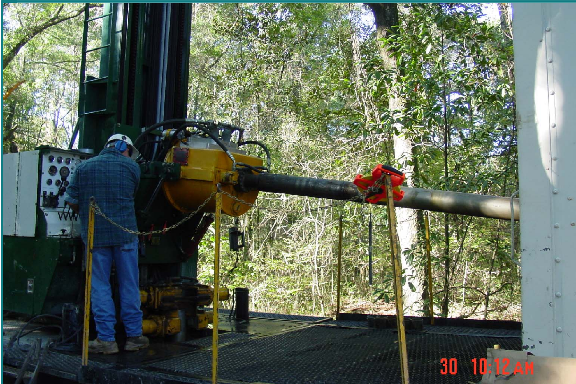
Photograph 5 Rotosonic Drilling Merritts Mill Pond Arsenic Study Marianna, Jackson County, Florida
