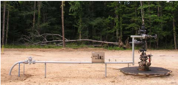
CO 2 -EOR production wellhead at a SECARB test site. (Courtesy: Bureau of Economic Geology, University of Texas–Austin)
