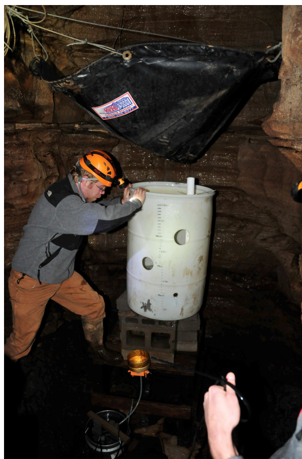
Figure 6. Barrel-shaped weir at Waterfall One in Crumps Cave for discharge measurements. Water level is measured with a pressure transducer in the barrel and the temperature, pH and spC probes are in the bucket below (photo by Jason Polk).
