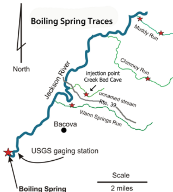
Figure 2. Sketch map showing the tracer tests to Boiling Springs. Small stars show location of sink points used for dye injection and large star is Boiling Springs (map by P.C. Lucas; 1 mile=1.6 km).
