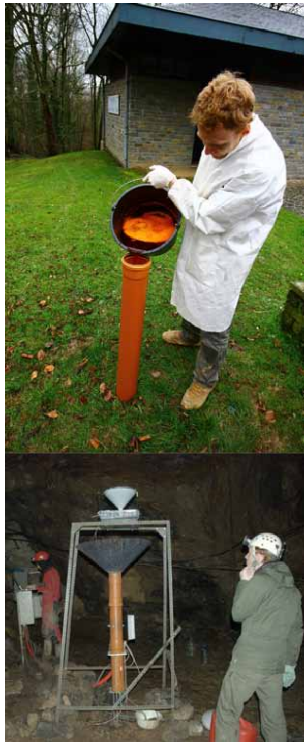
Figure 2. Injection of fluorescein above the cave with a PVC-pipe and a 40-liters flush of water. The monitoring is made of a Fluo-Green fluorometer above a drip water gauge.
