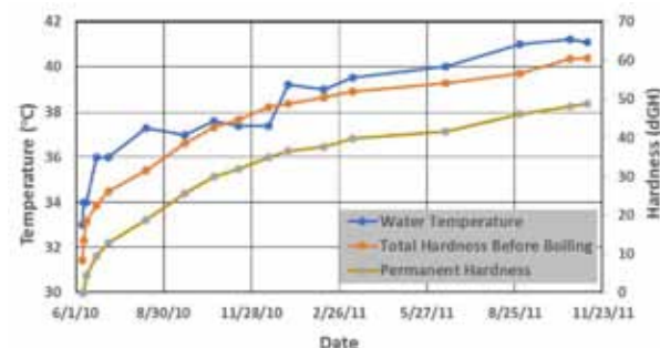
Figure 4. Water temperature and hardness measurements at borehole 4-3.
