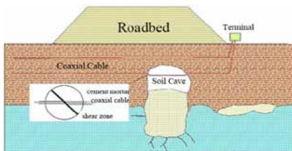
Figure 7. Schematic diagram of TDR monitoring technology for soil cave detection (Qin et al, 2010).
