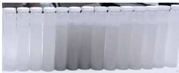
Figure 4. Visual turbidity change in Tippery Spring water samples capturing the storm pulse as it reached the spring. Increased turbidity resulted in darker bottles and therefore a lower pixel luminosity. Shown: May storm samples from 5/5/17 6:00–20:00.
