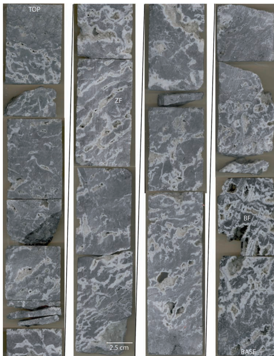
Figure 10. Core photographs from Whiteman #1 well, Chemung County, NY. This core has common fractures, vugs, zebra fabrics (ZF), boxwork fabric (BF) and an overall brecciated appearance. White saddle dolomite lines vugs and fractures in gray matrix dolomite. Core is 5 cm (2 inches) wide.
