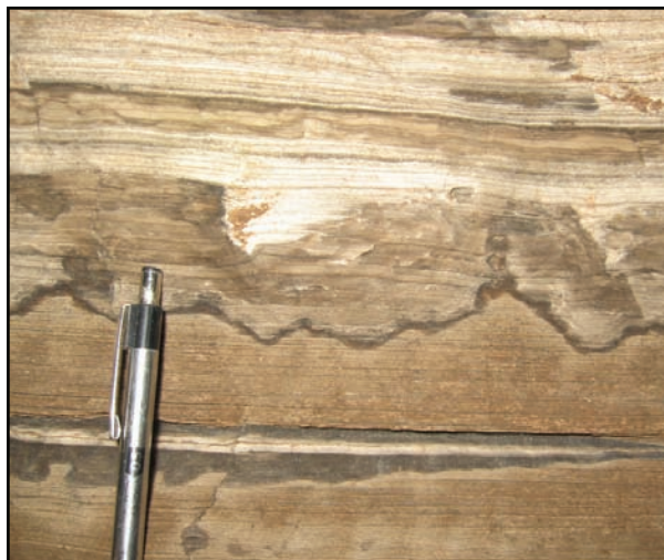
Figure 7. Diagenetic Boundary between gypsum and calcite. Darker, lower half is calcitized material. Note the boundary layer and continuation of varves from gypsum into calcite.
