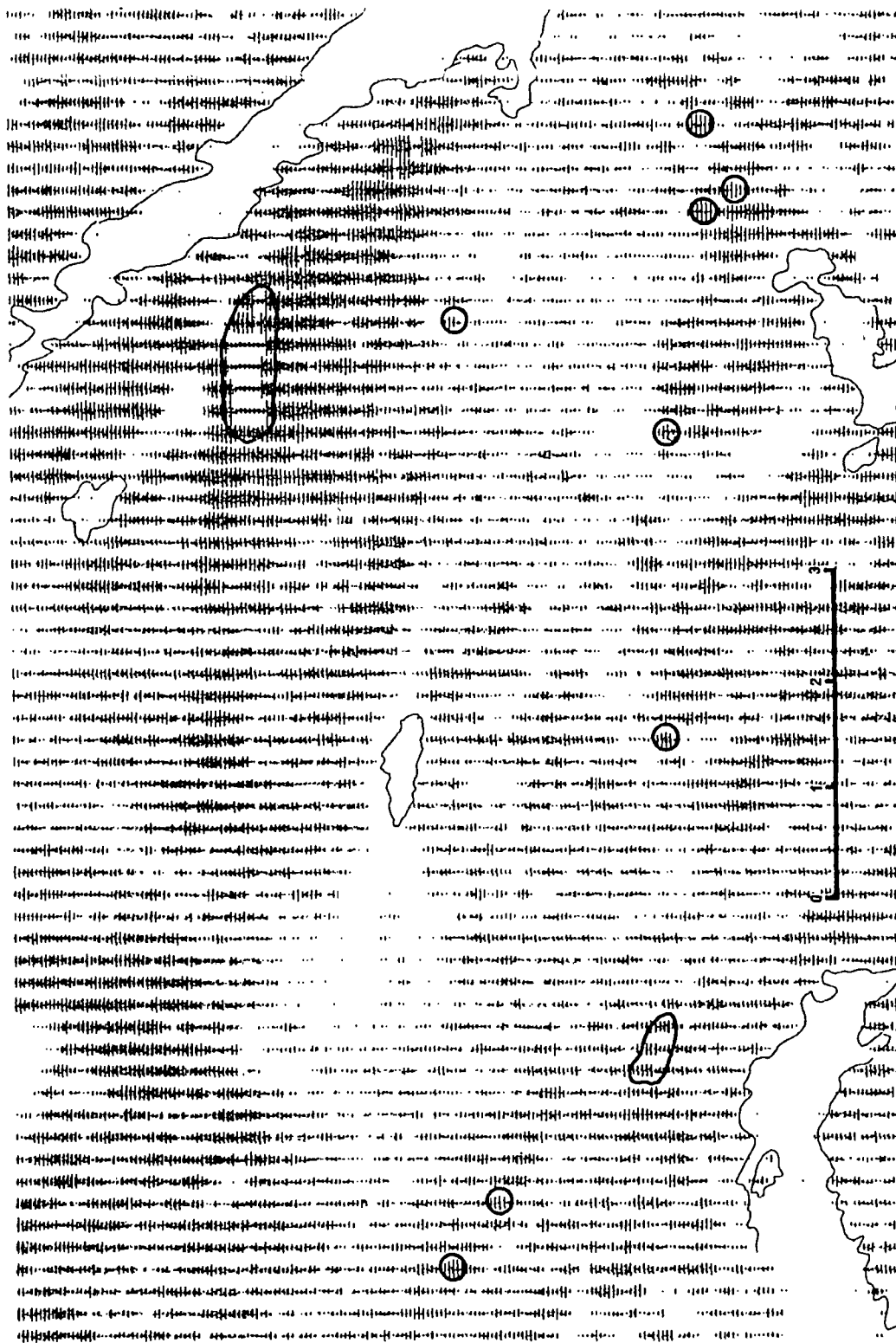
FIG. 9. Gamma spectrometric map of the area south of Söderhamn. Thicker grey lines = thorium. The +++ represents recordings of more than 15 ppm eU. Marked positions indicate field locations investigated in the follow-up of airborne measurements. Original scale 1:50 000. Measurements performed by Swedish Geological Co.
