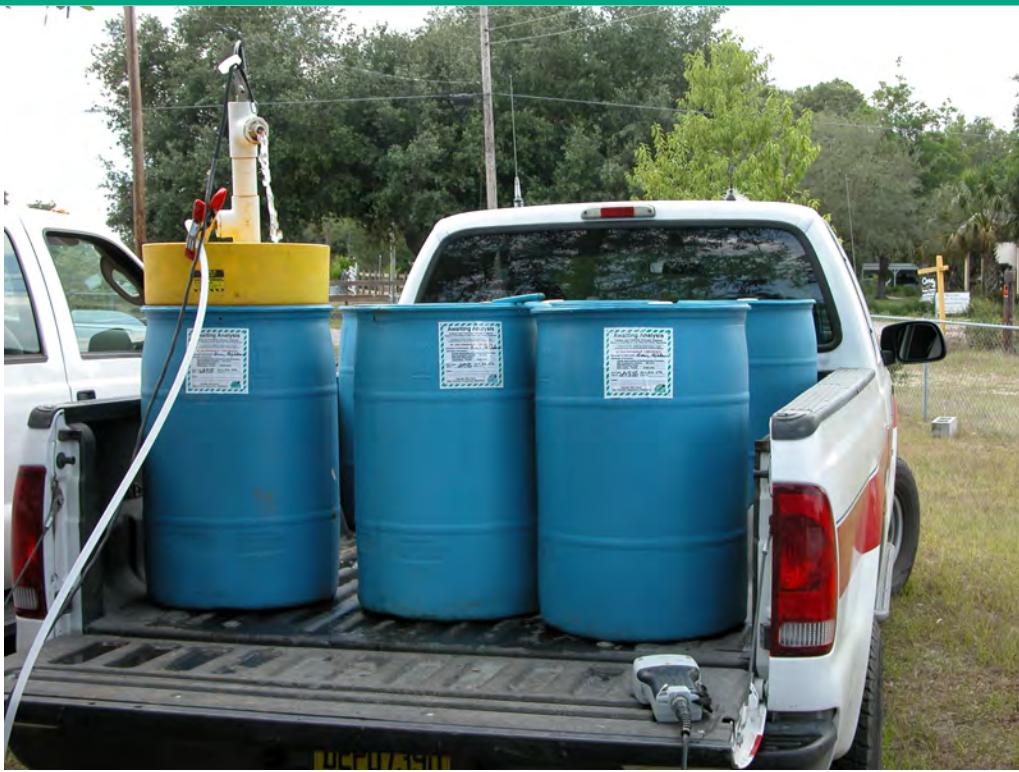
Containerizing Monitor Well Purge Water
