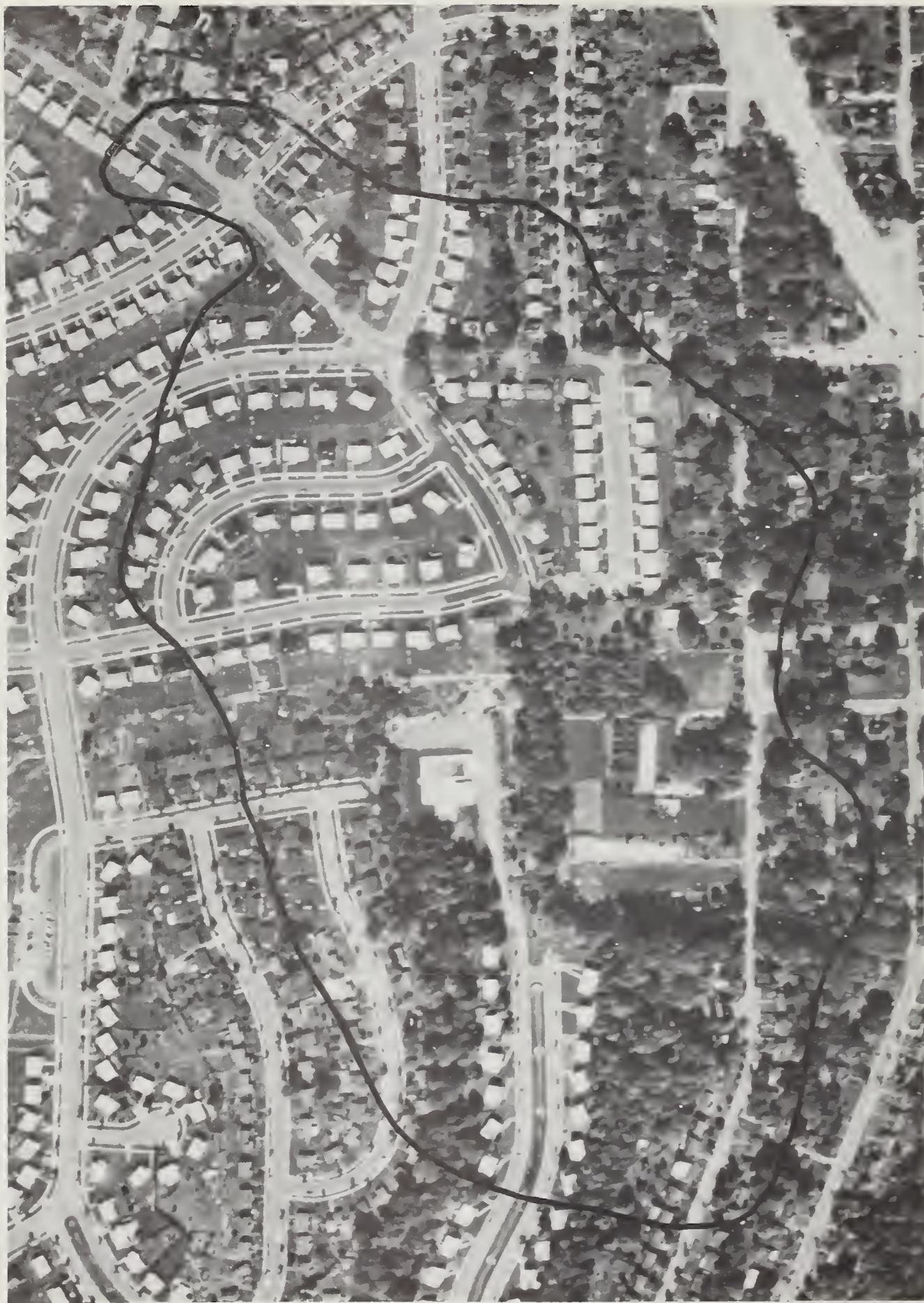
FIGURE 2. — Photograph taken May 7, 1961, on which the completed residential construction is shown. Stabilization of the construction area and the drainage channels caused a diminution of sediment outflow for many months. Scale, 317 feet per inch.
