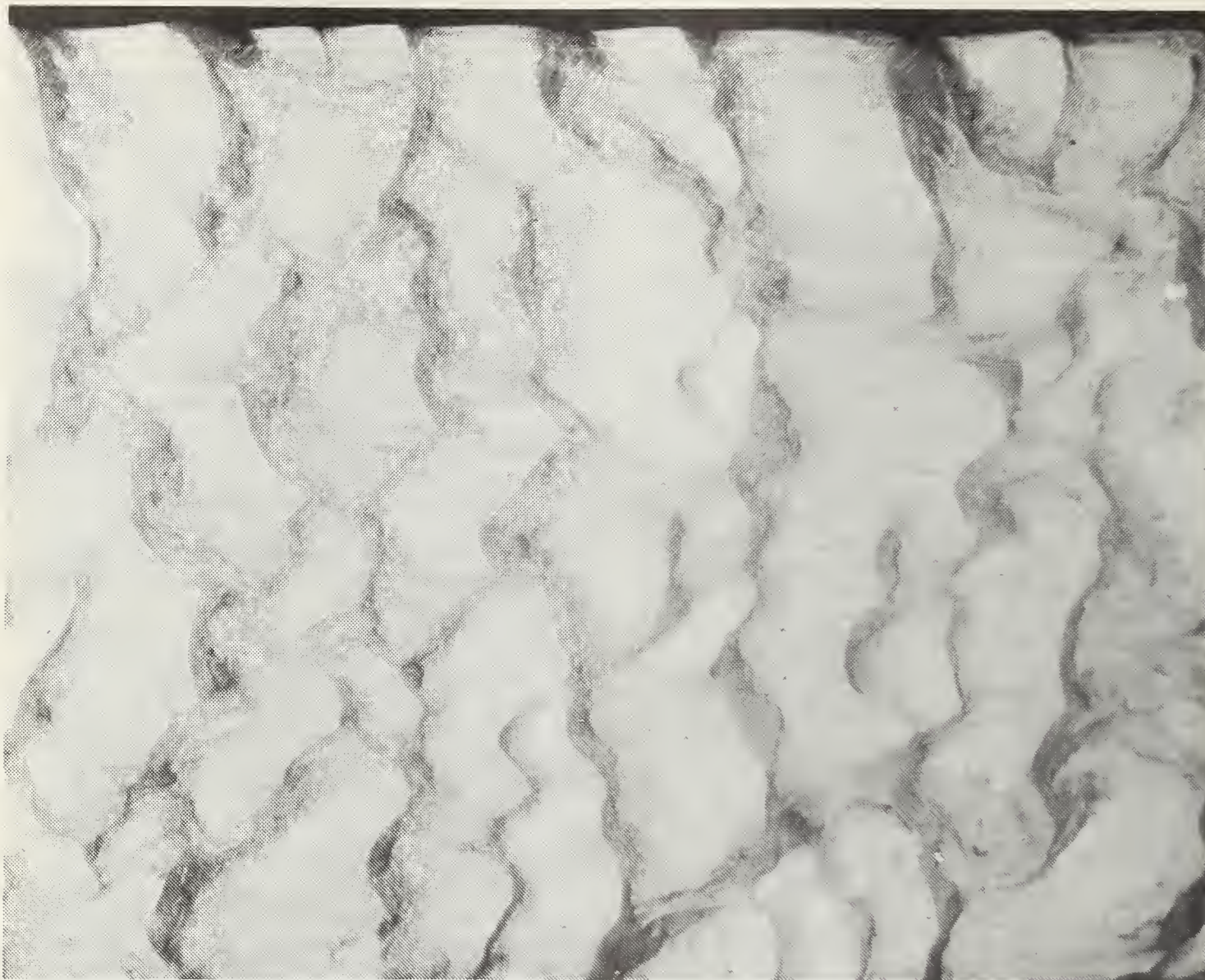
FIGURE 2. — Dune configuration of run 3-2. Flow direction left to right. Full 33.5-inch width of the flume is shown. Bed friction factor, f_b=0.102 .
