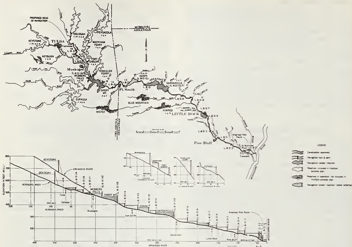
FIGURE 1.— General plan and profile of the multiple-purpose plan for the Arkansas River and tributaries in Arkansas and eastern Oklahoma.
