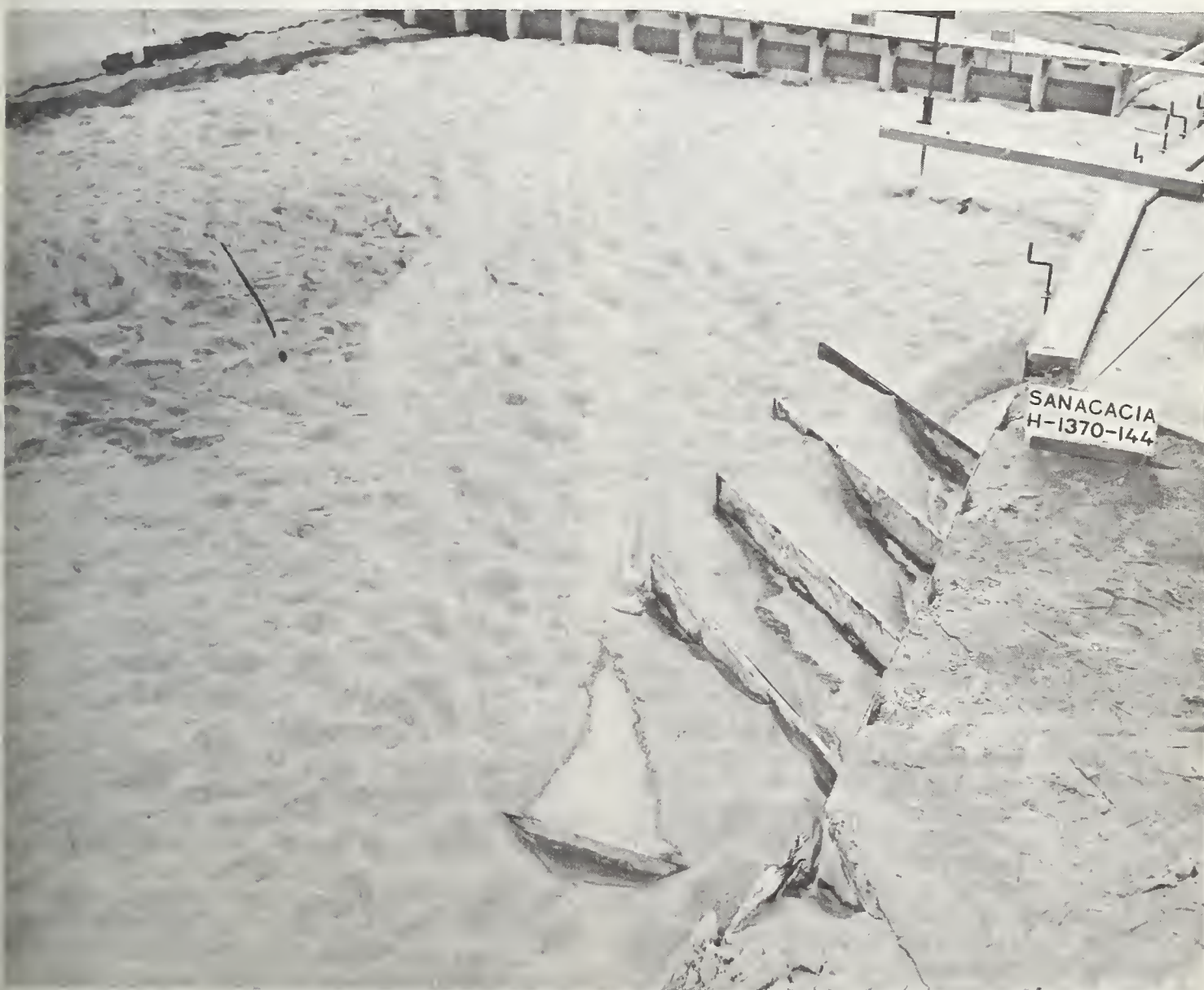
FIGURE 11. — Bottom vanes after test 18, showing sediment deposits partially covering vane area.
