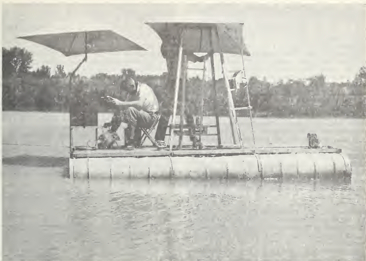
FIGURE 5.—Measuring the density of reservoir sediments. A dual probe, containing a radioactive source and a detection system, has been lowered from the raft into the sediment, and an activity density measurement is being made.
