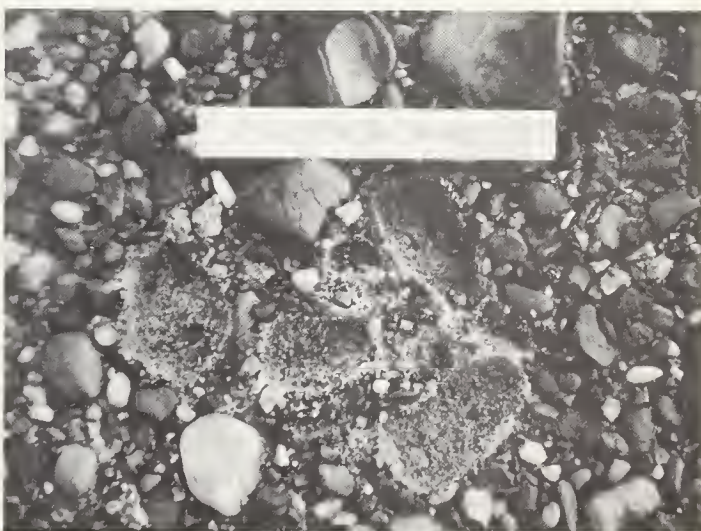
FIGURE 14. — Closeup view of bed surface armor, with several large gravel particles removed to show underlying sands.
