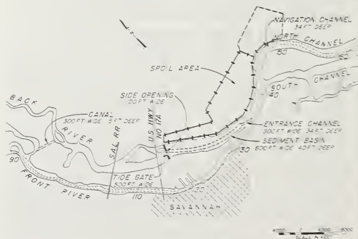
FIGURE 6.—Sediment basin with tide gate in downstream location (phase 8, scheme 6, test 4, and test 10).
