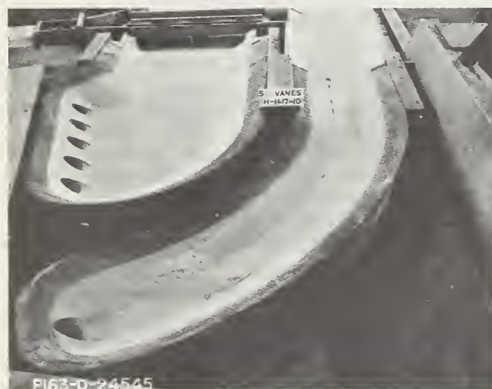
(b) Sediment Deposits in Canal After Test 21
