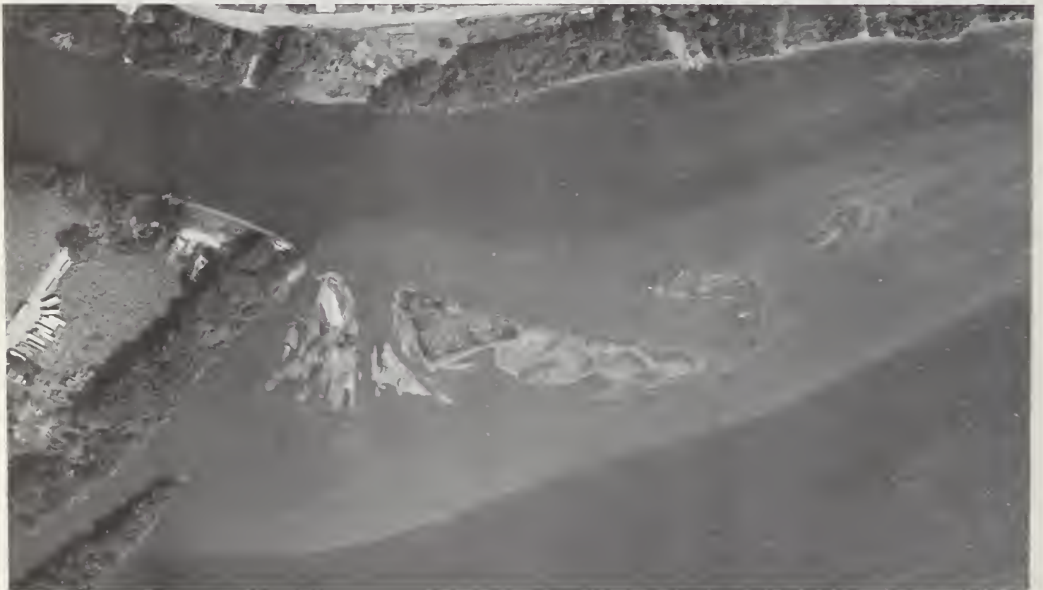
FIGURE 13. — Bars at Swatara Creek, September 15, 1961; discharge, 5,640 c.f.s.
