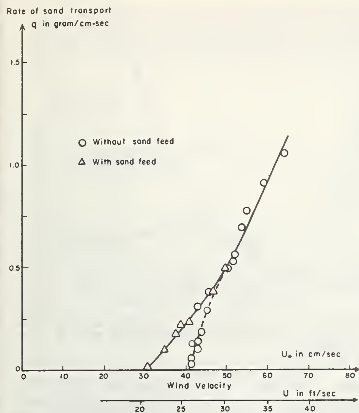
FIGURE 6.— Experimental data on the rate of transport of sand A ( d = 0.44 mm.) with and without a sand feed.
