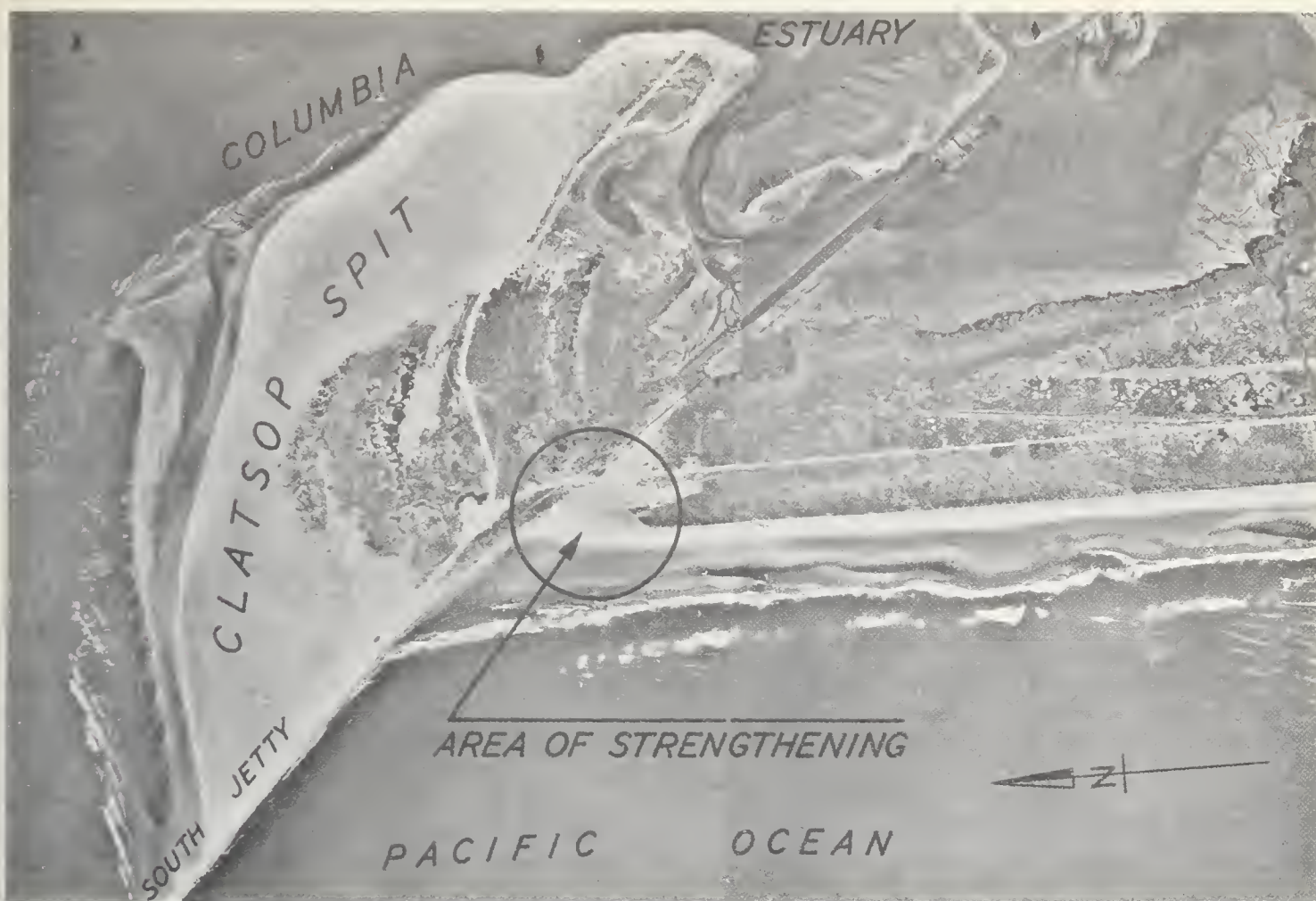
FIGURE 26. — Erosion south of South Jetty.
