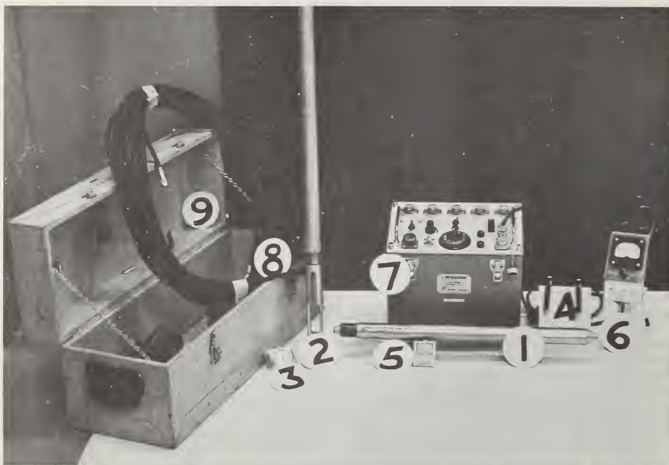
FIGURE 1. — A single gamma probe with operating accessories: (1) gamma probe containing the radioactive source, shielding, Geiger-Mueller detection tubes, and transistorized preamplifier; (2) aluminum connecting sections for inserting probe; (3) stopwatch; (4) personnel exposure pencils; (5) personnel exposure badge; (6) radiation meter; (7) portable scaler; (8) connecting cable; (9) carrying box, with lead shield, for gamma probe.
