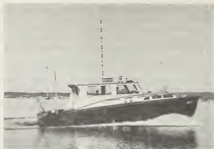
FIGURE 8. — Launch Dakota on Fort Randall Reservoir. Note stern sampling booms and antenna arrangement.
