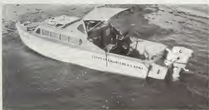
FIGURE 5.—Shallow draft cruiser used for independent sounding operations and transportation of the Raydist shore stations.
