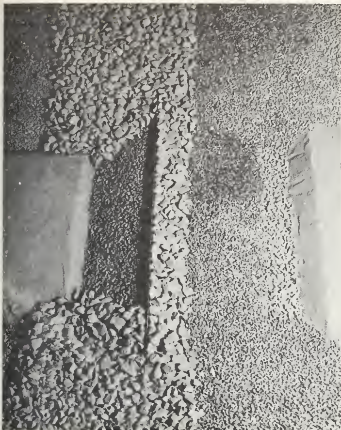
FIGURE 6.— Model sill after placement of filter and derrick stone. Flow will be from right to left.
