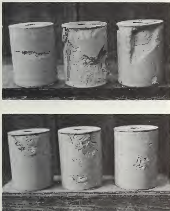
FIGURE 6. — Typical scour patterns.
