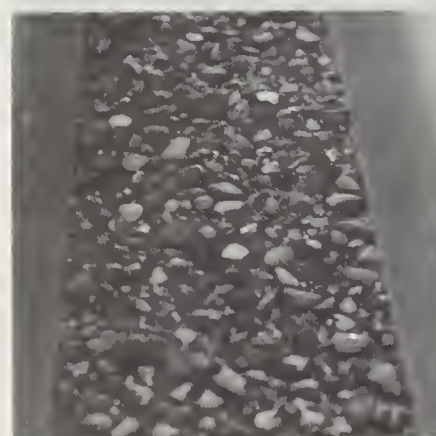
FIGURE 9. — Changes in bed characteristics during scour, as observed by A. S. Harrison in a flume study conducted at the University of California.
