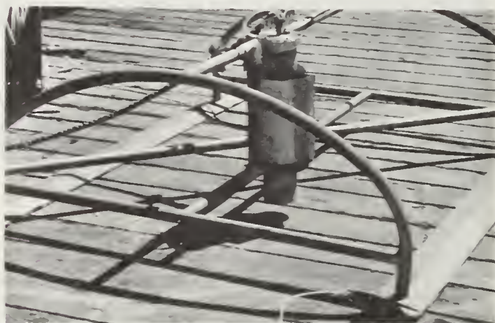
FIGURE 6. — Radiation detector mounted on sled.
