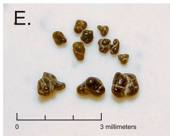
Figure 3. Photomicrographs of Aquia aquifer sediments: A. Washed sand. B. Quartz grains: iron-stained (left), clear (right). C. Calcite: cement (left), shell fragments (right). D. Goethite grains. E. Glauconite grains. Sample from well CA Db 96, 580 to 600 feet.
