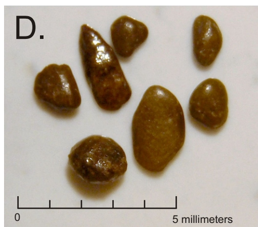
Figure 3. Photomicrographs of Aquia aquifer sediments: A. Washed sand. B. Quartz grains: iron-stained (left), clear (right). C. Calcite: cement (left), shell fragments (right). D. Goethite grains. E. Glauconite grains. Sample from well CA Db 96, 580 to 600 feet.
