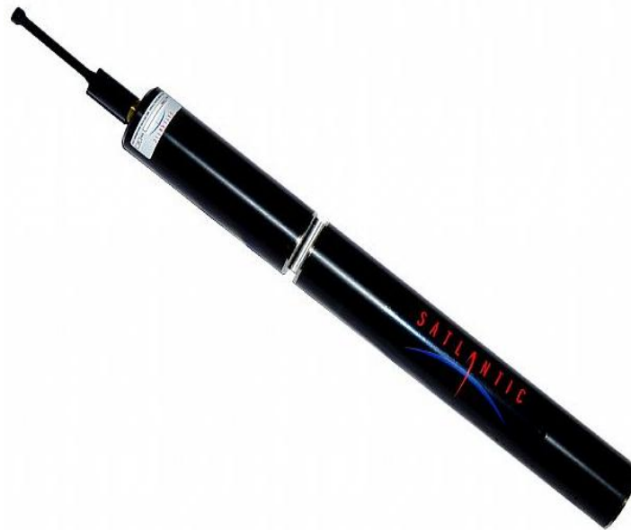
Fig. 2-2 – Photograph of the Satlantic Submersible UV Nitrate Analyzer (SUNA). Data communications occur via the port to the upper left; the sensor requires off-board power and data storage, and is therefore tethered during the entirety of each deployment. The UV-lamp irradiates across the 1-cm gap 1/3 rd down the sensor, passing through the ambient fluid; no flow cell was used during our deployments. A copper guard was inserted in the sensor gap to preclude biofilm development. In addition, the sensor was wrapped in Nitex mesh to prevent benthic invertebrate colonization. Power and data cables were reinforced using garden hoses to prevent impacts from turtles and other herbivores. (Photo Credit: http://www.satlantic.com/photos/513000_Plastic%20SUNA.jpg )
