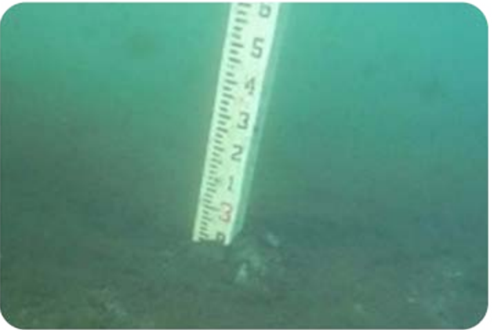
Organic sediment accumulation in the upper Homosassa River is caused by particulate material settling out from the water column as flow declines. Sediment thickness can be as much as 4 feet thick in the upper reaches of the river.
