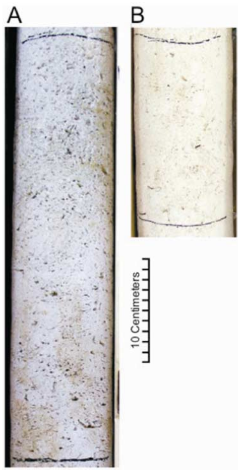
Figure 2. Photographs of limestone core samples (a) 18 and (b) 30. Both limestone cores are examples of matrix porosity from a test core hole adjacent to production well S-3168 at the Northwest well field [see Renken et al. , 2008, Figure 1]. Core sample 18 was taken from interval depth of 6.0–6.3 m. Core sample 30 was taken from interval depth of 13.7–13.9 m. Note the greater visible (secondary) porosity in core 18 versus core 30.
