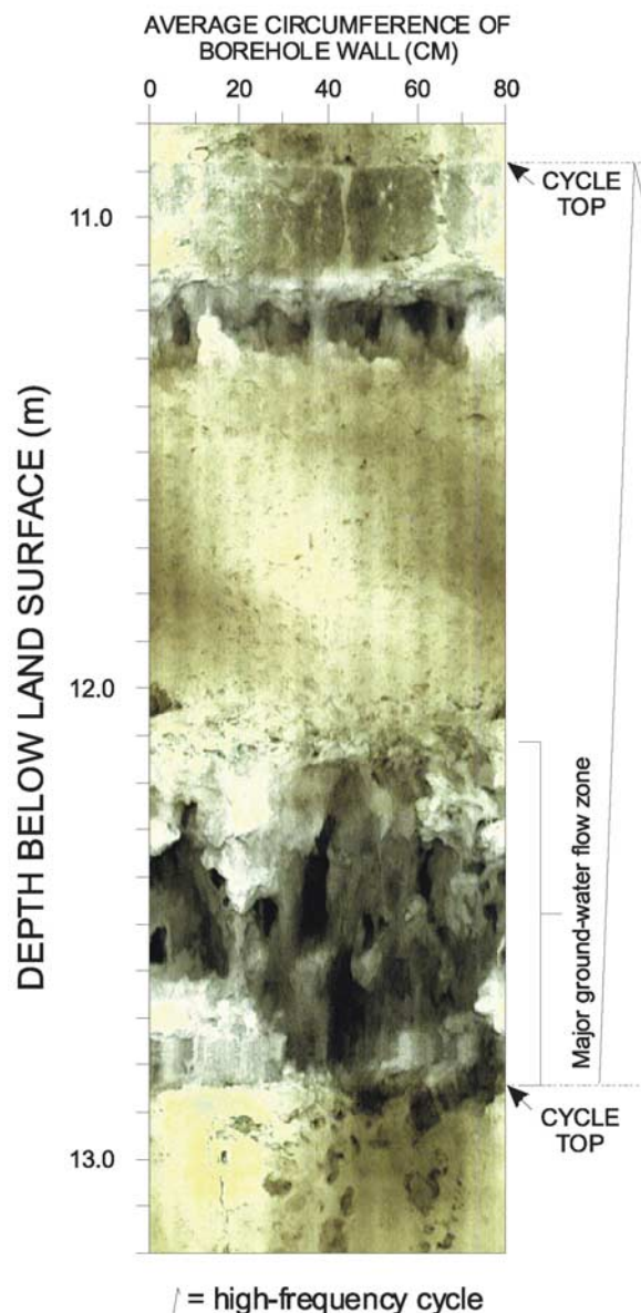
Figure 3. Digital image of the borehole wall that spans the injection interval in injection well G-3816 [see Renken et al. , 2008, Figure 1]. Note the major groundwater flow zone near the base of the injection interval with a pore system characterized by touching-vug porosity and overlying limestone with a pore system mainly characterized by matrix porosity [Cunningham et al. , 2006a, 2006b]. Injection well G-3816 is a horizontal distance of 1 m from injection well G-3817.
