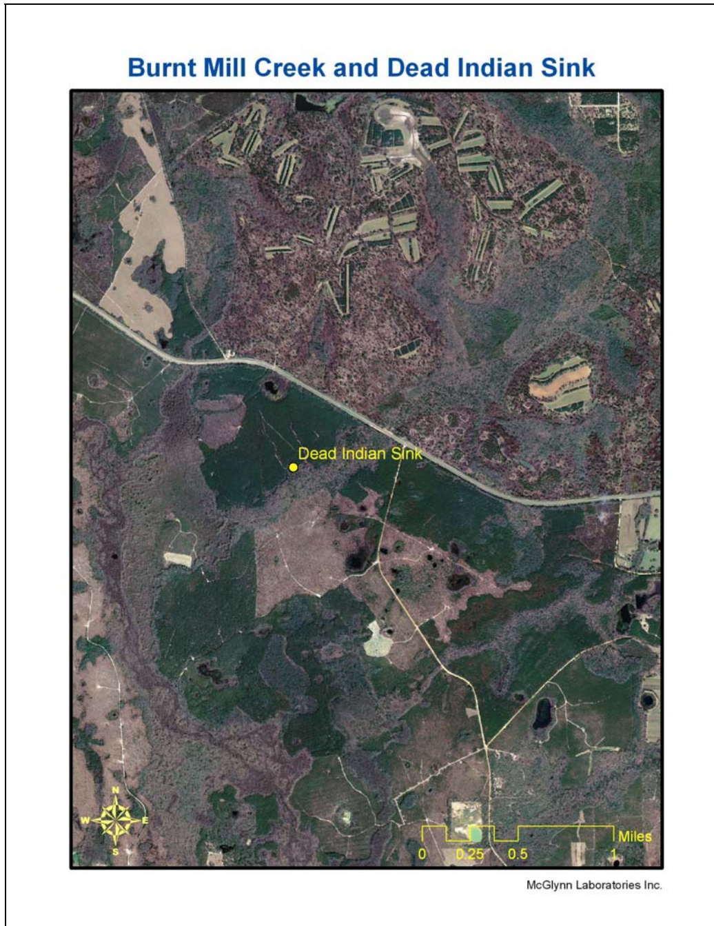
Figure 1.3.18: The location of the dye injection and sensor placement for the fourth dye study from Dead Indian Sink where Burnt Mill Creek sinks into the aquifer to the St. Marks Rise. Dead Indian Sink is approximately 10 miles from the St. Marks Rise.
