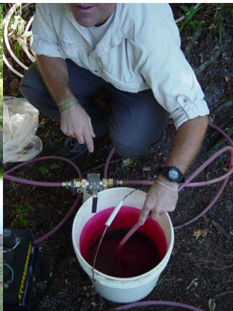
Figure 1.3.9: Injecting dye and pumping it to the cavern.
