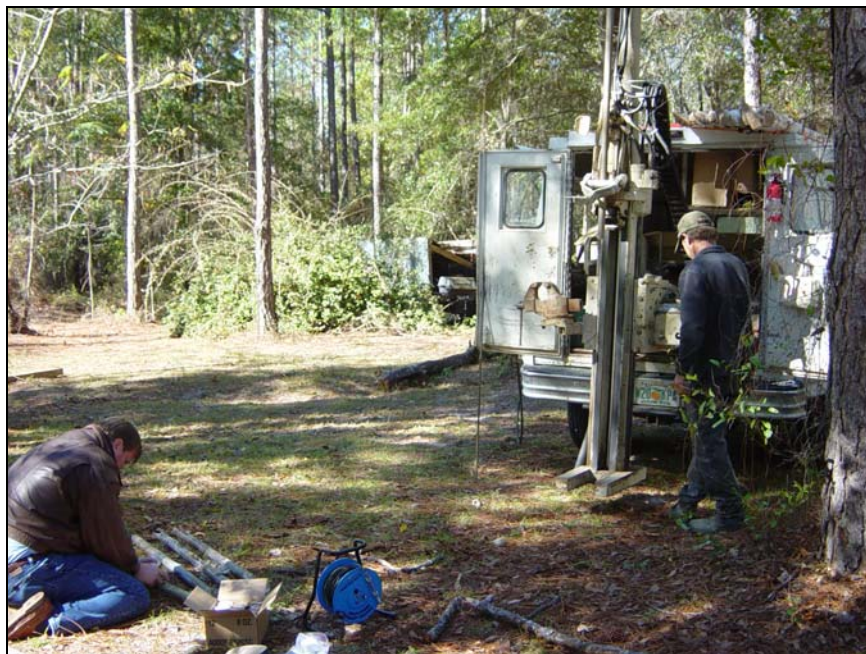
Figure 1.1.11: Coring into the top of the aquifer. Steve Reece of Ardaman and Associates sampled the cores. JD Kemp Geological Investigations installed the wells.
