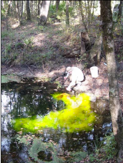
Figure 1.3.14: Injecting the dye in the sink at Rhodes Spring #2
