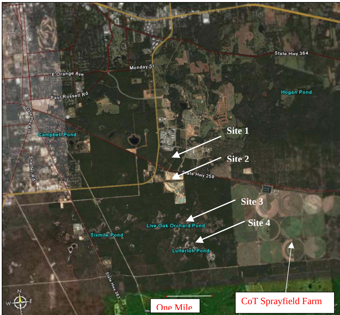
Figure 3.6: map depicting the sites shown in the following pictures. Site 2 was where the new sinkholes formed. Sites 1, 3 and 4 are altered natural features, mostly karst in nature, that are part of the Shepards Branch Drainage.
