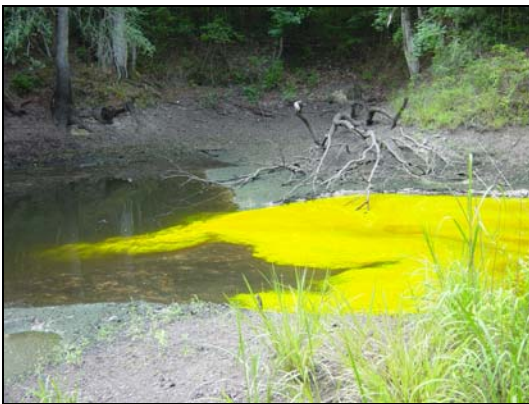
Figure 1.3.23: Rhodamine wt dye, 1 kg, was poured into Burnt Mill Creek on July 22, 2006 at 17:20
