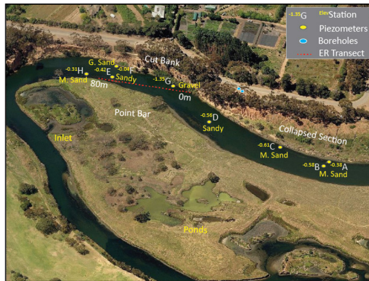
Figure 3.2. In-stream piezometer stations and ER transect line. Piezometer labels indicate the sediment substrate. Ponds on the point bar can be seen east of the piezometer locations.
