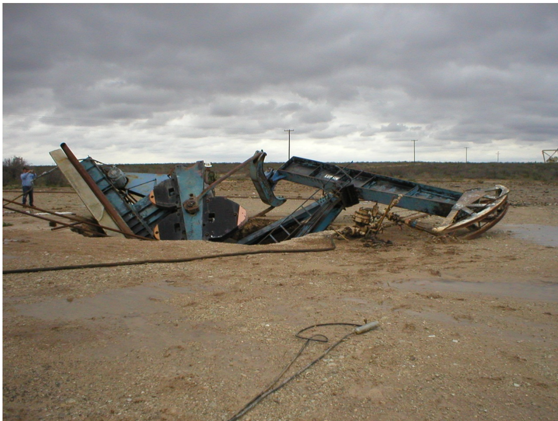
Figure 12. Pump jack in sinkhole, Dagger Draw oil field, Eddy Co., New Mexico.
