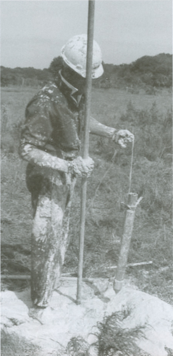
Geophysical technician installs a 5-pound explosive charge into a shothole.
