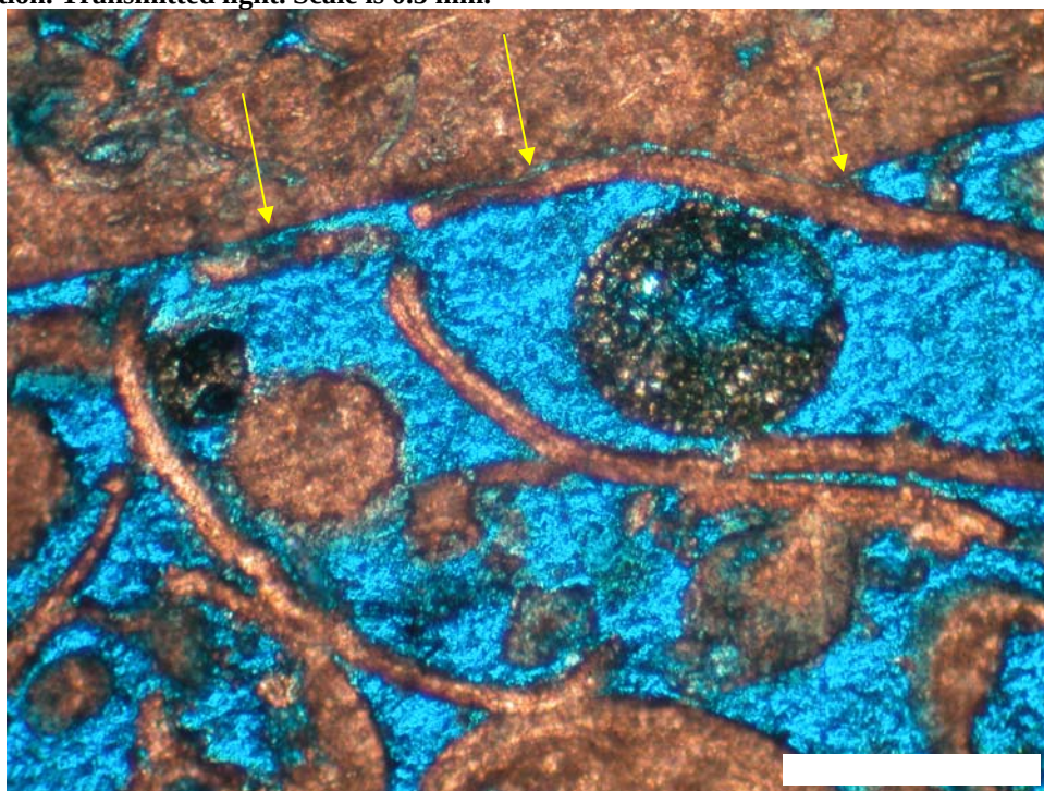
Figure 71. W-18778, 995-996. Highly micritized, foraminiferal, grainstone. Close up view showing edge (arrows) of the large mold (Figure 68). Inside the mold is very low-mud with some grain breakage and not much compaction. The very fine crystalline green-black circular area is possibly an artifact of making the thin section. Plane polarized light. Scale is 0.25 mm.
