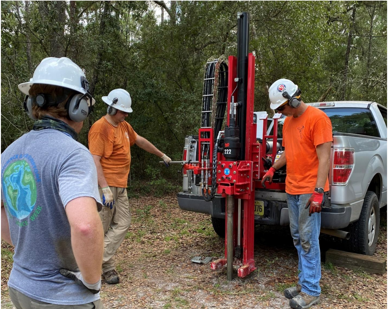
Figure 4. FGS staff geologists running the DPT rig an AMS 9120 RAP Power Probe TM , in Ralph E. Simmons State Forest.
