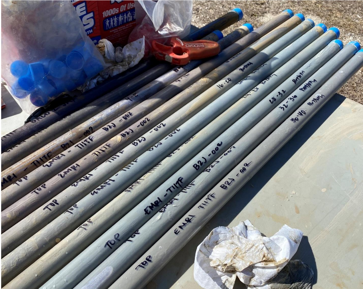
Figure 5. Samples collected using direct push technology. These samples were collected using the equipment in Figure 4, a truck mounted rig capable of collecting 1.5-inch diameter samples in 4-foot runs.
