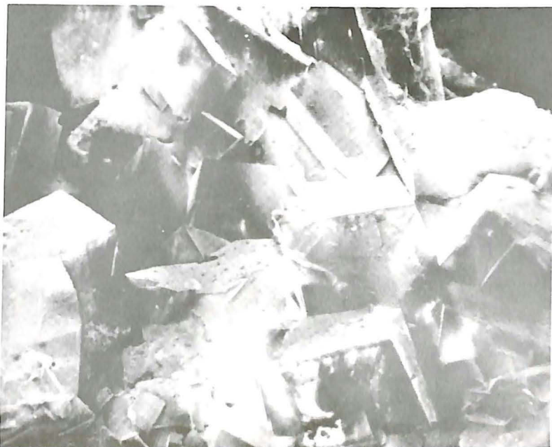
Figure 56 Scanning Electron Microphotograph of dolomite, medium crystal sucrosic, euhedral, 20% vugs and intragranular porosity, Eo-3 (depth 3440 - 3500 ft.), Mobil No. 1 Babcock Ranch (Well 10), Charlotte County (X100).
