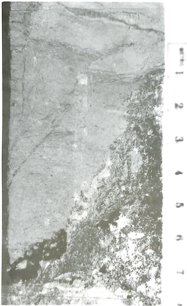
Figure 37 Photograph of the top of the dolomite zone at 2046 feet in U. S. Gypsum Core (Well 30) showing peaty partings and limestone in irregular contact with incompletely dolomitized limestone.
