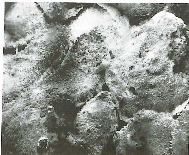
Figure 44 Scanning Electron Microphotograph of Skeletal limestone from Unit Eo-2, 100% coarse grained (depth 2435 - 50 ft.), Gulf-Cal. Block 46 (Well 46) Monroe County (X100).
