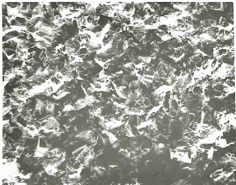
Figure 54 Scanning Electron Microphotograph of dolomite, fine crystalline, euhedral, Tampa Stage (depth 1035 ft.), Coastal No. 1 State Monroe County (X100).
