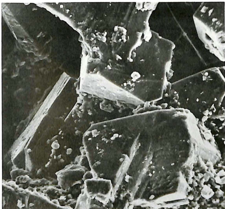
Figure 28 Same as Figure 27, enlarged X1500 showing faces of crystals and intergranular porosity.
