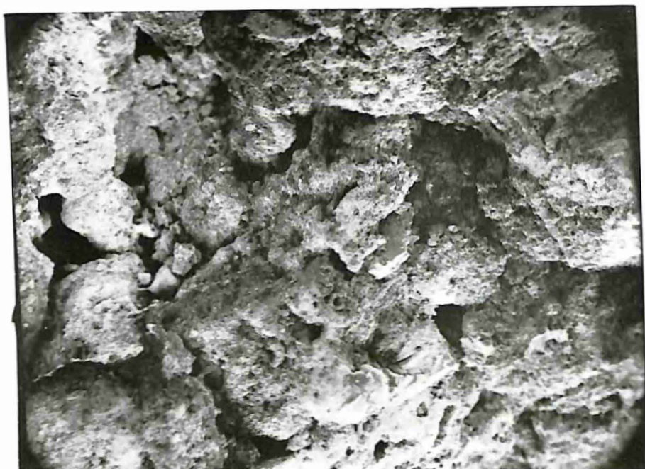
Figure 46 Scanning Electron Micrograph of Skeletal limestone from Tampa Stage (depth 1160 - 70 ft.), Co stal No. 1 State (Well 52) Monroe County (X100).
