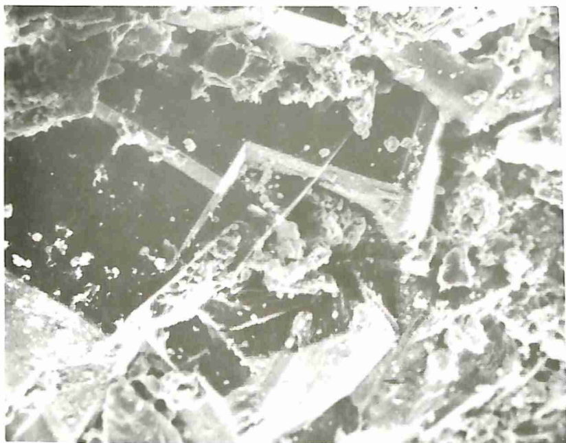
Figure 55 Same enlarged X1000 to show faces of dolomite crystals.
