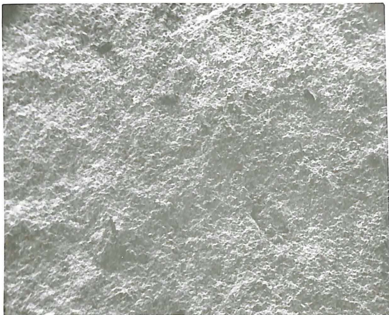
Figure 50 Scanning Electron Microphotograph of lithographic dolostone from Unit Eo-3 (depth 3540 - 50 ft.), Coastal No. 1 State (Well 52) Monroe County (X100).
