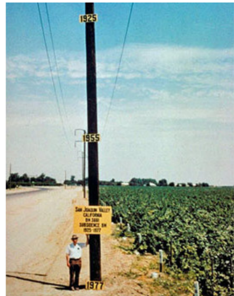
Figure 19. Fifty years of subsidence (over 20 feet) in California's San Joaquin Valley. Image courtesy of National Geodetic Survey (NGS).
