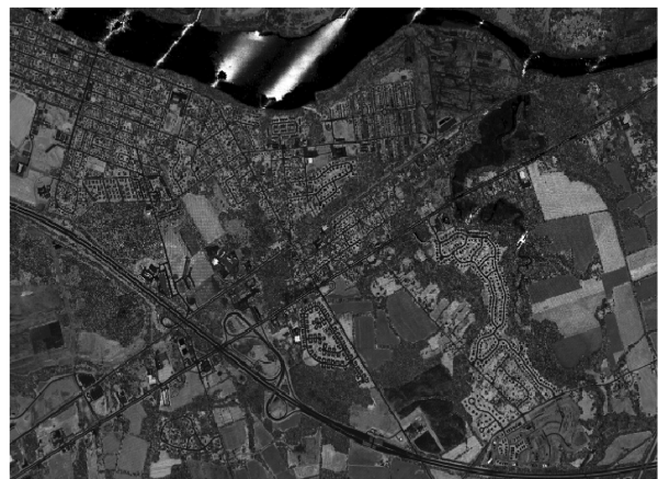
Figure 27. Intensity image showing streaks over water from multiple flight lines. This is not a problem because topographic LiDAR measurements on water are already assumed to be unreliable and are classified separately as LAS Class 9.
