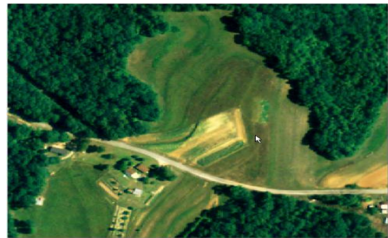
Figure 47. Color orthophoto doesn't reveal topographic characteristics clearly visible in the prior figure.
