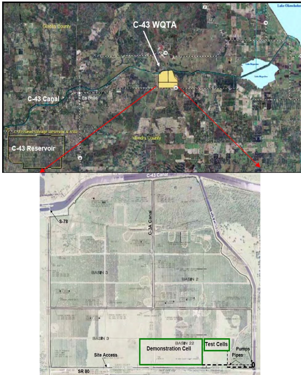
Exhibit 1 - Location of the C-43 Water Quality Treatment and Demonstration Project (top panel) and layout of the test and demonstration cells (bottom panel). (CH2M HILL 2009).
