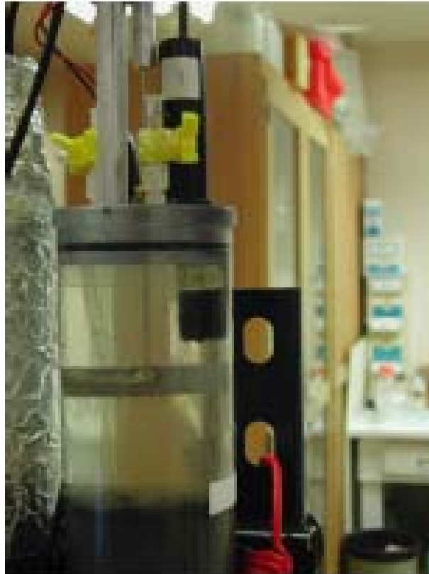
Core Incubator: end cap showing oxygen electrode, stirring motor, stirring paddle, sampling ports, and sample withdrawal tube (Val Klump et al. , 2004)
