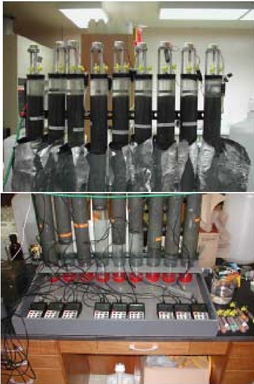
Core Incubator: setup for simultaneous run of nine cores. Cores are covered with aluminum foil during incubation. Also shown are oxygen electrodes (Val Klump et al. , 2004).
