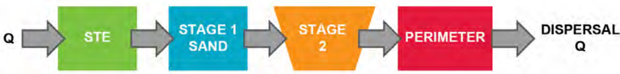
Figure 16. Example Flow Diagram: In-Ground Stacked Biofilter, Single Pass Stage 1 Over Stage 2 Lignocellulosic (Hazen and Sawyer 2015b)
