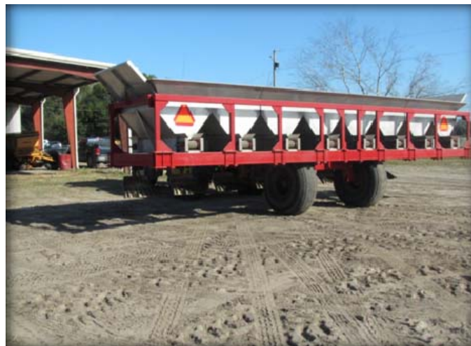
FIGURE 29: AGRICULTURE FERTILIZER BANDING EQUIPMENT FOR EIGHT ROWS
