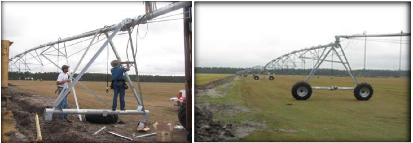
FIGURE 18: OVERHEAD PIVOT IRRIGATION ON SOD WITH FERTIGATION
