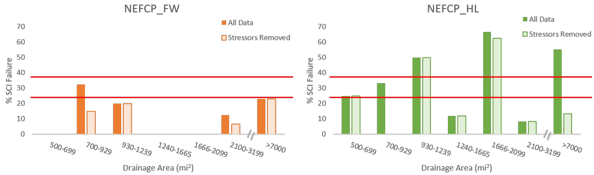
Figure 12. Percent SCI failure versus drainage area (mi 2 ) for NEFCP Flatwoods (left) and Highlands (right) after stressor removal. Red lines indicate estimated thresholds of unacceptable SCI failure rates.
