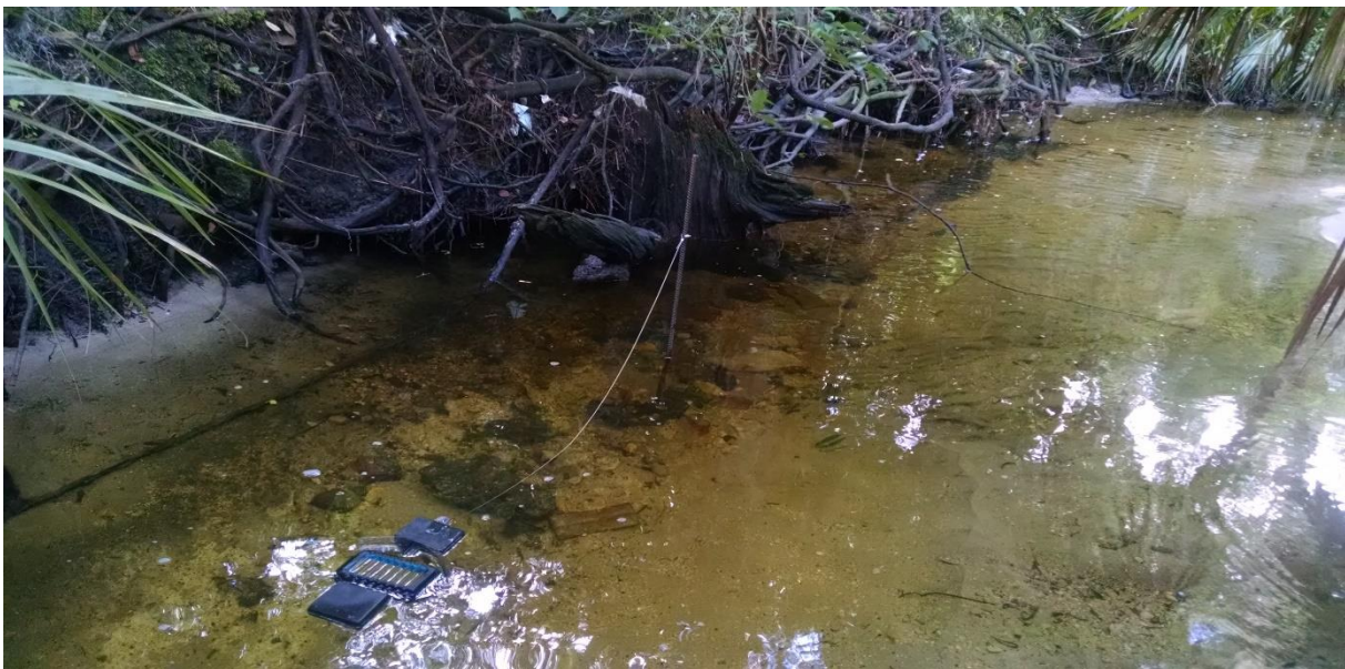
Figure 3-9. Sweetwater Branch downstream of KGS during periphyton rack retrieval from the only pool found in the 100 m reach (reflecting sediment smothering).
