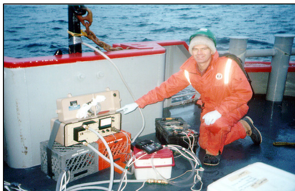
Fluorometric Sampling. The fluorometer is a device that provides on-site measurements and tracking of polynuclear aromatic hydrocarbons (PAH) in the water column (Figures 15 and 16).
