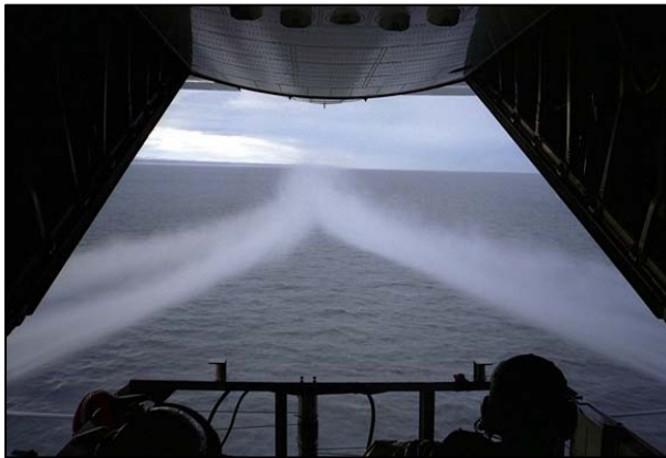
Figure 8. ADDS Pack spray seen from inside
