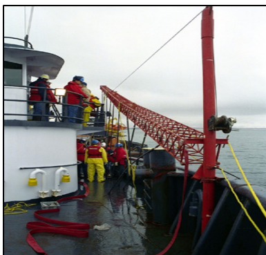
Figure 13. Deployment of spray arms
