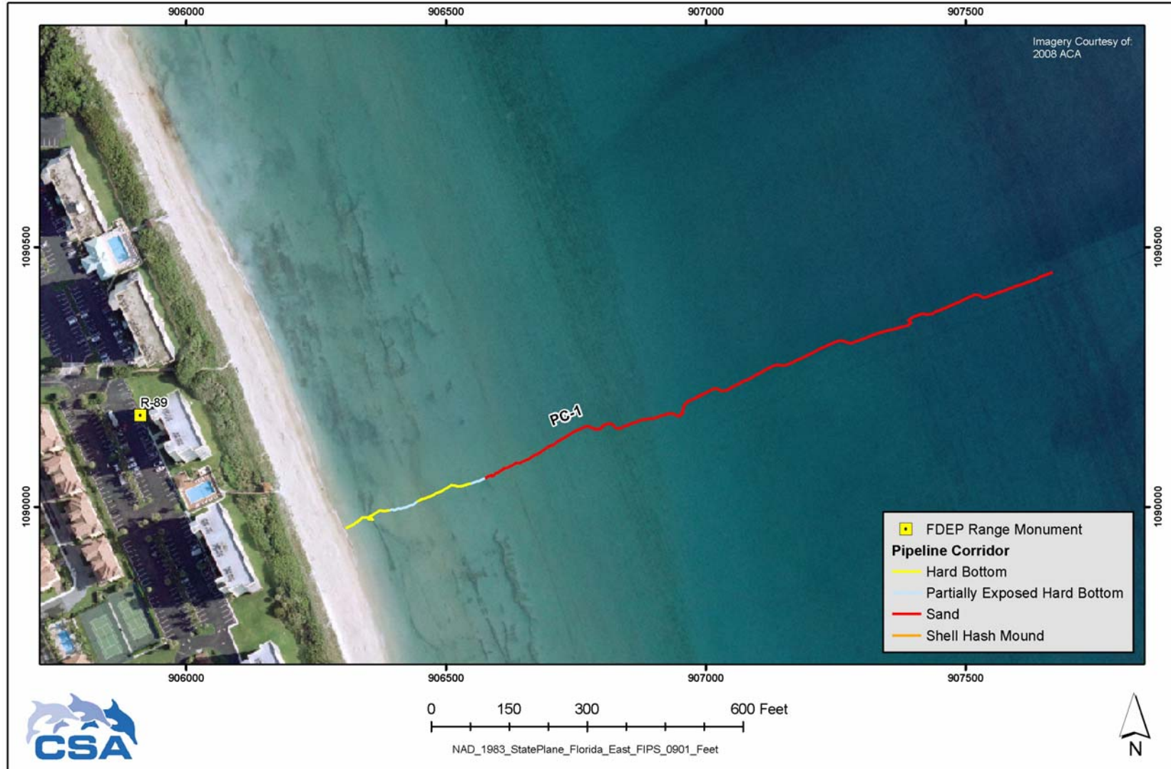
Figure D-33. Potential pipeline corridor PC-1 near FDEP Range Monument R-89 mapped during the Baseline Nearshore Hard Bottom Characterization Survey for the St. Lucie County South Beach Project. Yellow lines denote hard bottom, blue lines denote partially exposed hard bottom, and red line denotes sand. Geo-referenced qualitative video data were collected along the entire proposed pipeline corridor. Survey conducted 16 July 2009.
