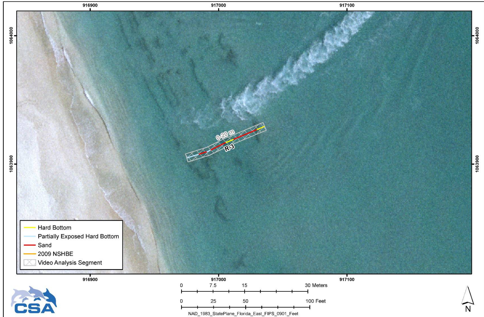
Figure D-22. Transect R-3 established during the Baseline Nearshore Hard Bottom Characterization Survey for the St. Lucie County South Beach Project. Yellow lines denote hard bottom, blue lines denote partially exposed hard bottom, red lines denote sand and/or shell hash gaps, and orange line denotes mapped nearshore hard bottom edge (NSHBE). Box indicates the transect segment selected for video analysis. Hard bottom survey conducted 15 August 2009.
