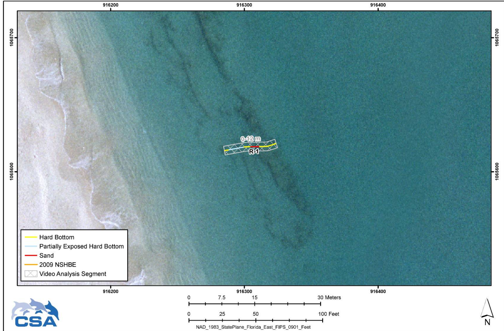
Figure D-21. Transect R-1 established during the Baseline Nearshore Hard Bottom Characterization Survey for the St. Lucie County South Beach Project. Yellow lines denote hard bottom, blue line denotes partially exposed hard bottom, red line denotes sand and/or shell hash gaps, and orange line denotes mapped nearshore hard bottom edge (NSHBE). Box indicates the transect segment selected for video analysis. Hard bottom survey conducted 15 August 2009.
