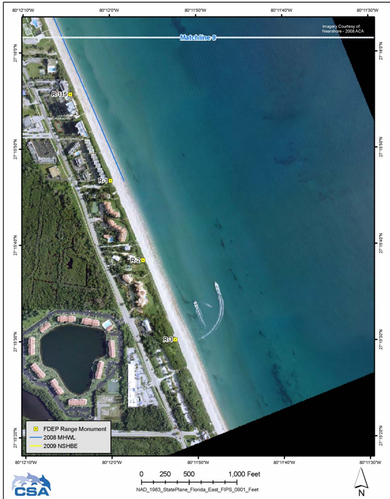
Figure D-32. Overview of the nearshore hard bottom edge (NSHBE) between FDEP Range Monuments R-115 and R-3 mapped during the Baseline Nearshore Hard Bottom Characterization Survey for the St. Lucie County South Beach Project.
