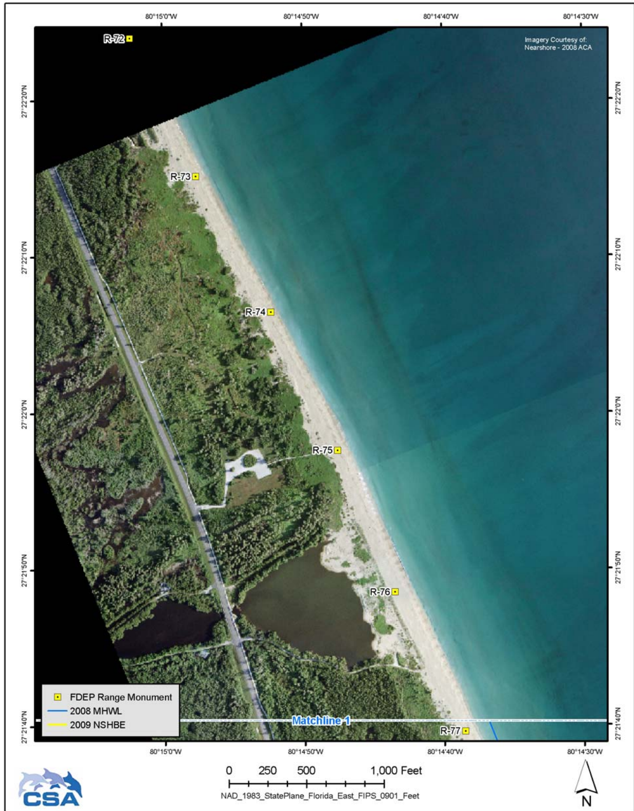
Figure D-23. Overview of the nearshore hard bottom edge (NSHBE) between FDEP Range Monuments R-73 and R-77 mapped during the Baseline Nearshore Hard Bottom Characterization Survey for the St. Lucie County South Beach Project.
