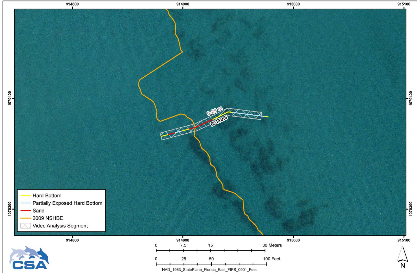
Figure D-19. Transect R-110.5 established during the Baseline Nearshore Hard Bottom Characterization Survey for the St. Lucie County South Beach Project. Yellow lines denote hard bottom, blue lines denote partially exposed hard bottom, red lines denote sand and/or shell hash gaps, and orange line denotes mapped nearshore hard bottom edge (NSHBE). Box indicates the transect segment selected for video analysis. Hard bottom survey conducted 15 July 2009.
